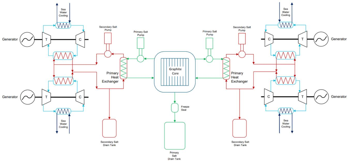
Figure 5 – Proposed diagrammatic plant layout.
