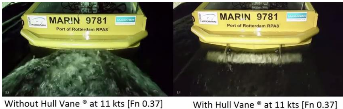
Figure 7: Demonstration of Hull Vane stern wake reduction (Van Oossanen Naval Architects, 2020)
