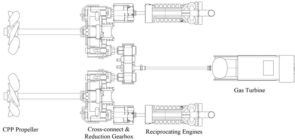
Figure 5: CODOG Propulsion System Layout
