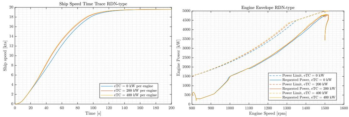
Figure 8: Results for the acceleration manoeuvre with the RDN approach, showing the ship speed (left) and the requested power plotted in the engine envelope (right) for different PTI settings
