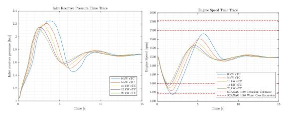
Figure 4: Simulation results of inlet receiver pressure(left) and engine speed (right) for a step load 200 kW-385 kW and different PTI power settings
