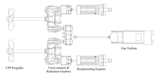
Figure 5: CODOG Propulsion System Layout
