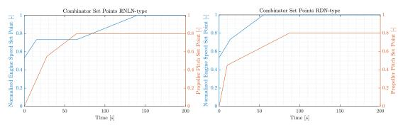
Figure 6: Combinator Set Points for Engine Speed and Propeller Pitch as used by the Royal Netherlands Navy (RNLN,left) and the Royal Danish Navy (RDN,right)
