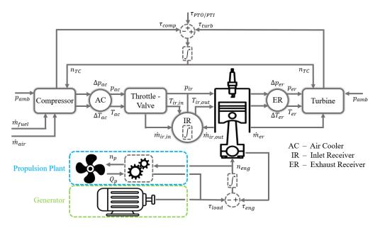
Figure 1: Block diagram of the proposed simulation model showing the reduction in volume elements involved in the gas exchange process and the investigated use cases with propulsion plant and generator.
