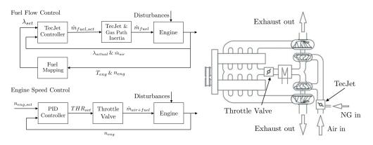
Figure 2: Schematic layout of the engine and controller from [54]
