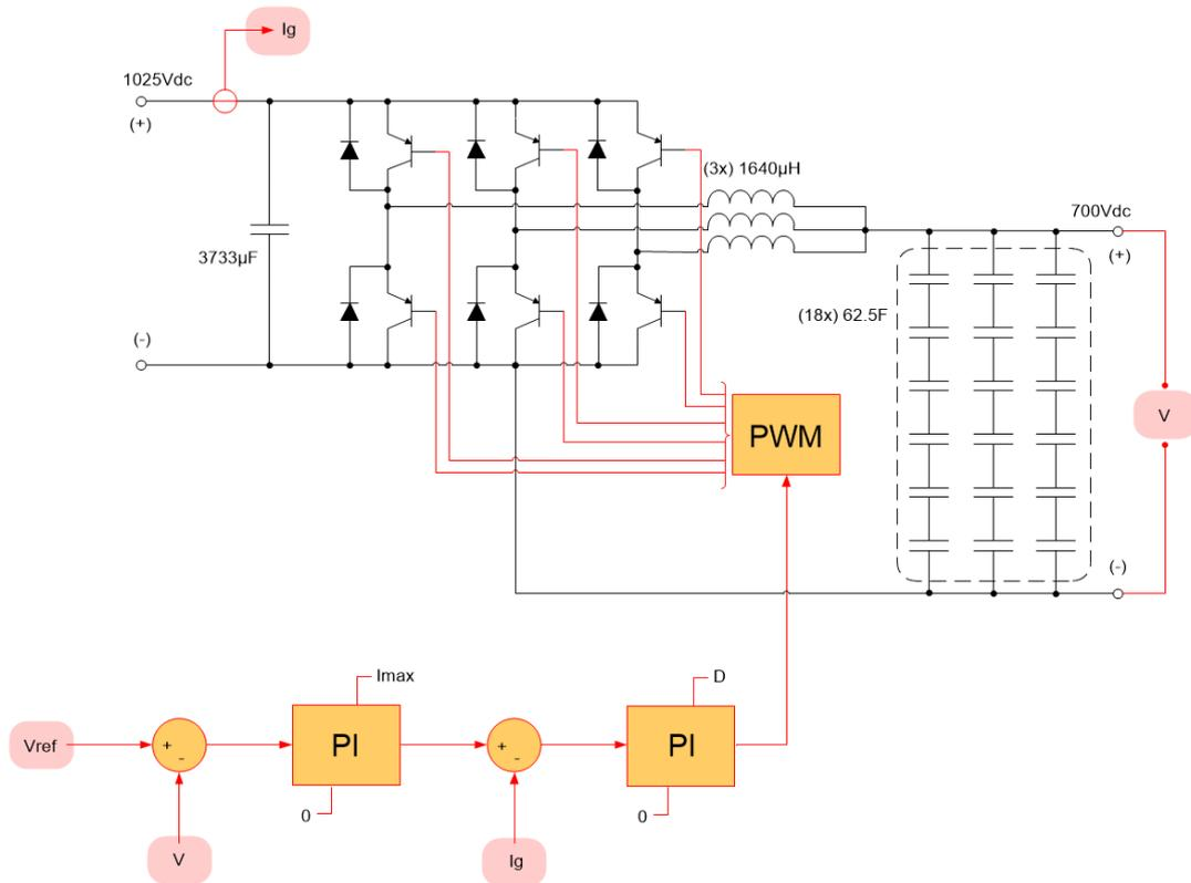
Figure 6: Zonal primary chopper converters (1025/700 V) controlling representation
