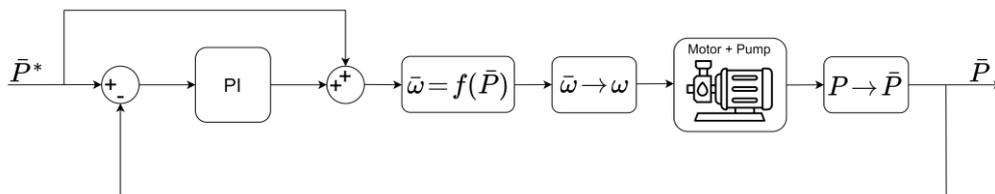
Figure 13: Pump motor control feedback loop
