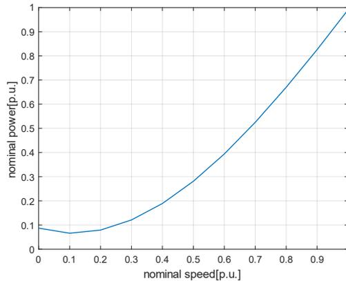
Figure 11: Nominal pump speed vs. power curve
