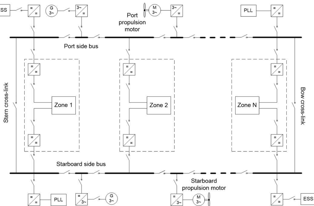
Figure 1: SLD representation of a shipboard power system based on ZEDS (Deroualle & Vinks, 2024)
