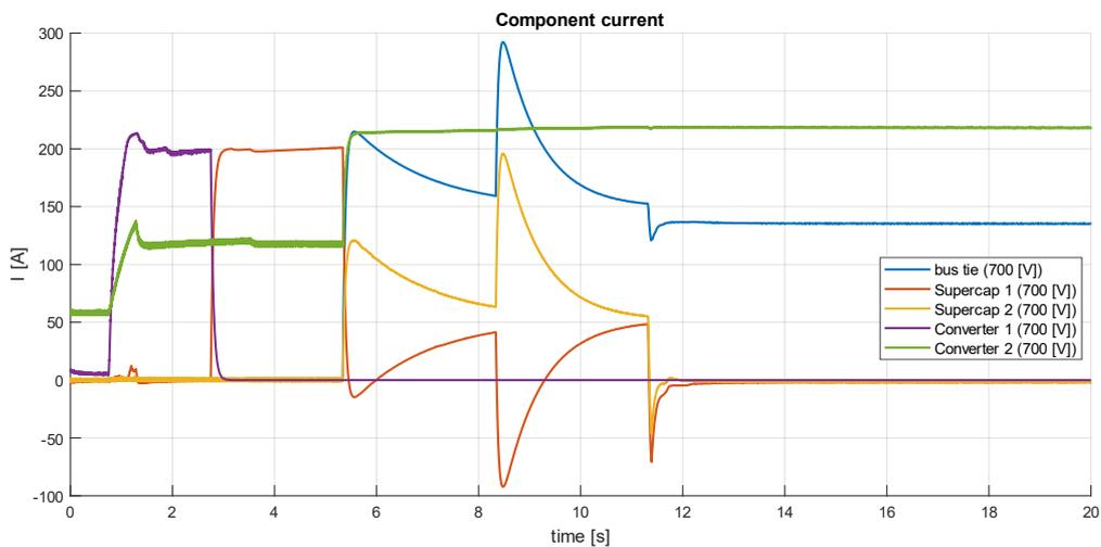
Figure 16: Power system components' current over time
