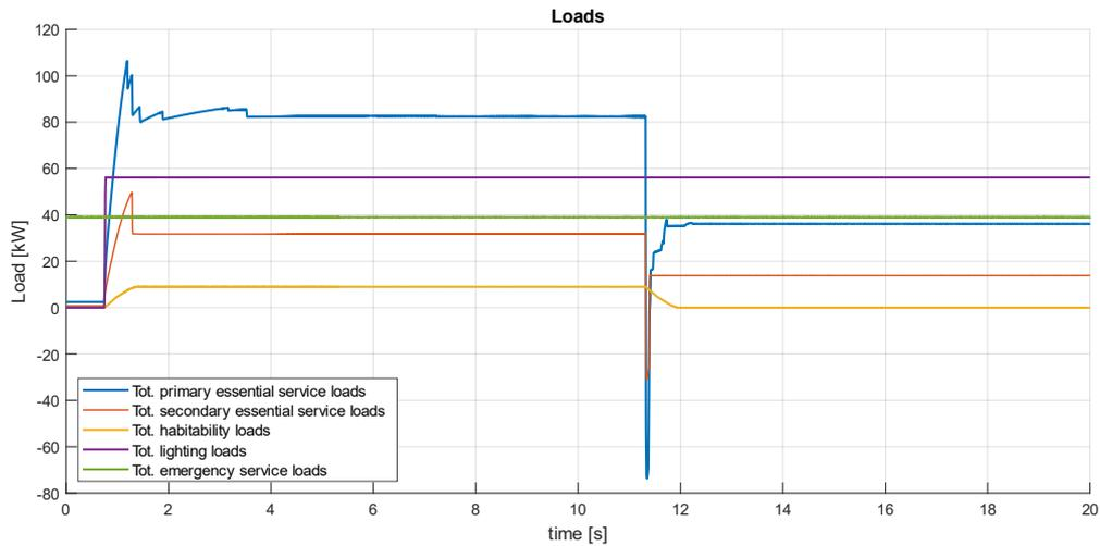
Figure 15: Service level component load sums over time
