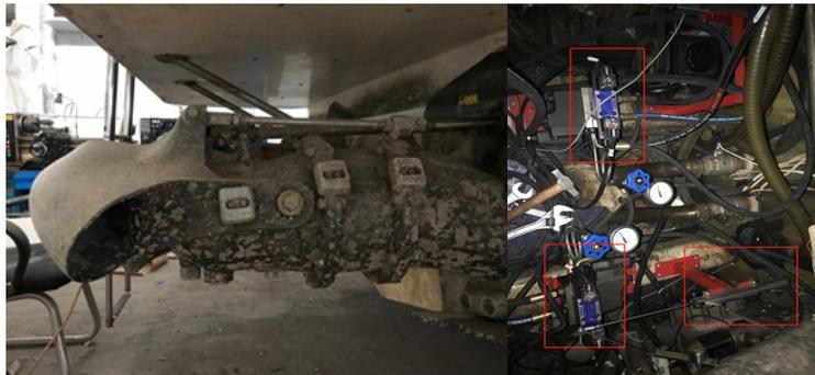
Figure 11: The reversing bucket and its structures (left) and The solenoid valve and electronic ruler (right).
