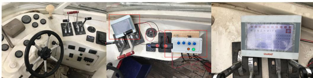
Figure 9: the control cabin: the steering wheel(left), the manned control table(middle), and the touch screen(right).
