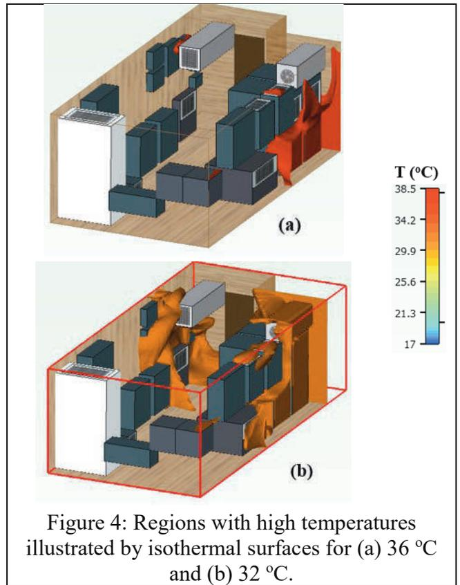
Localized hotspots are the major indicator of the failure of the cooling system to draw out hot air from the supply region of the cabinets. This is observed by streamlines (colored by temperature) in Figure 5 where due to short-circuiting of cold air, a large amount of cold air bypasses the IT equipment and replaced by surrounding hot air.
