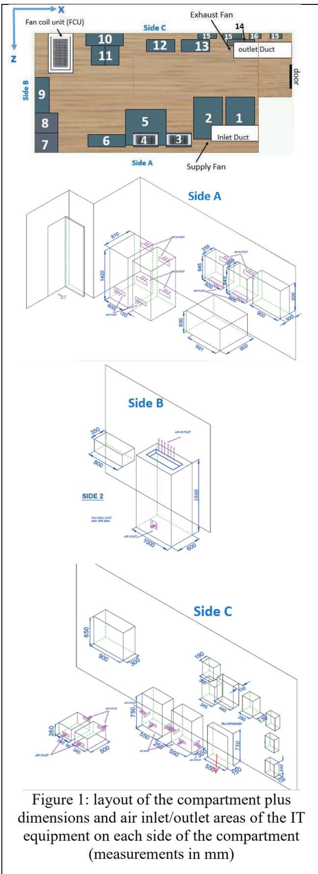
Figure 1: layout of the compartment plus dimensions and air inlet/outlet areas of the IT equipment on each side of the compartment (measurements in mm)
