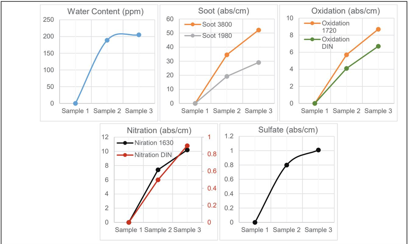
Figure 6: Different oil properties of three oil samples measured using standard laboratory based techniques
