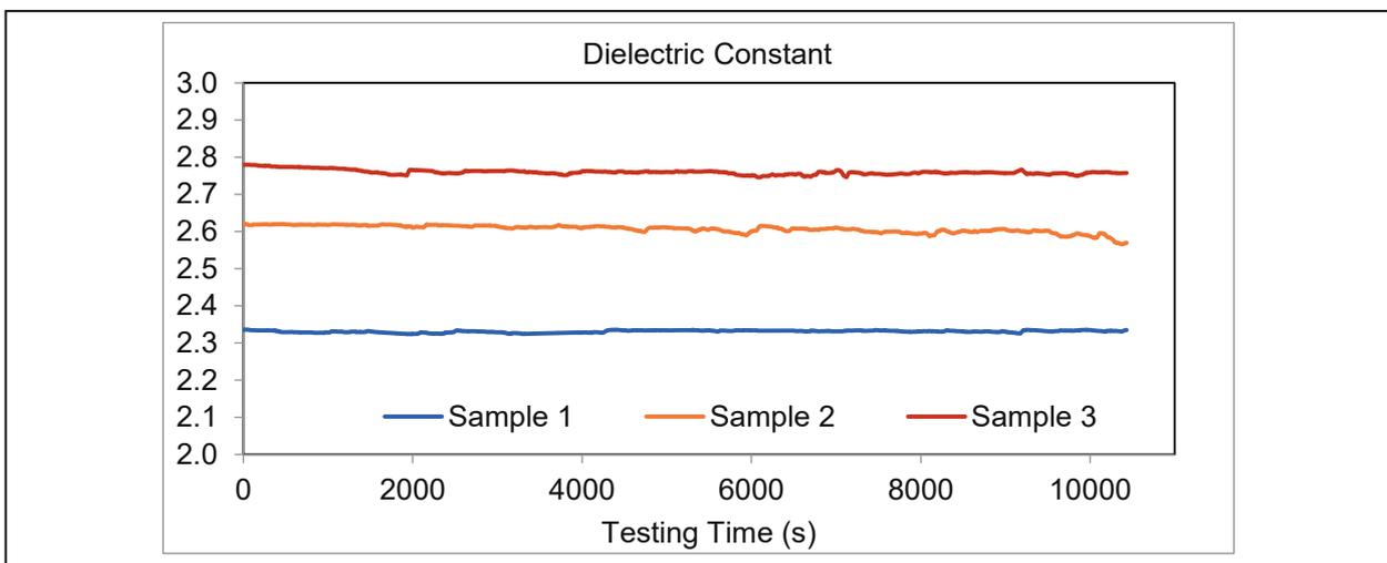
Figure 5: Typical representative curves of dielectric constant vs time for three oil samples measured using oil sensor
