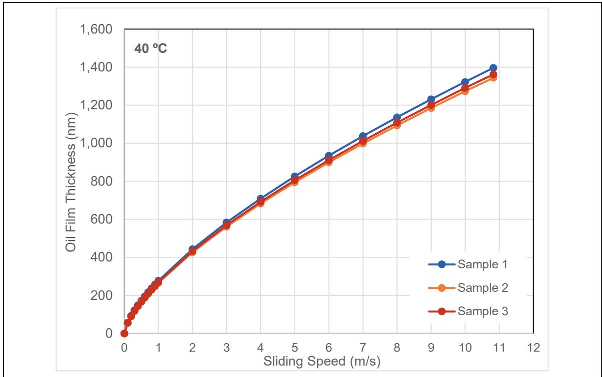
Figure 3: Minimum oil film thickness formed by three lubricating oil samples at 40 °C
