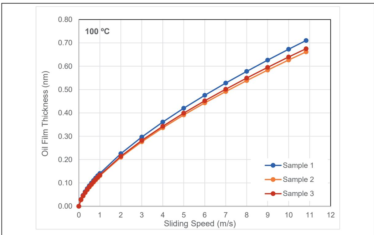
Figure 4: Minimum oil film thickness formed by three lubricating oil samples at 100 °C
