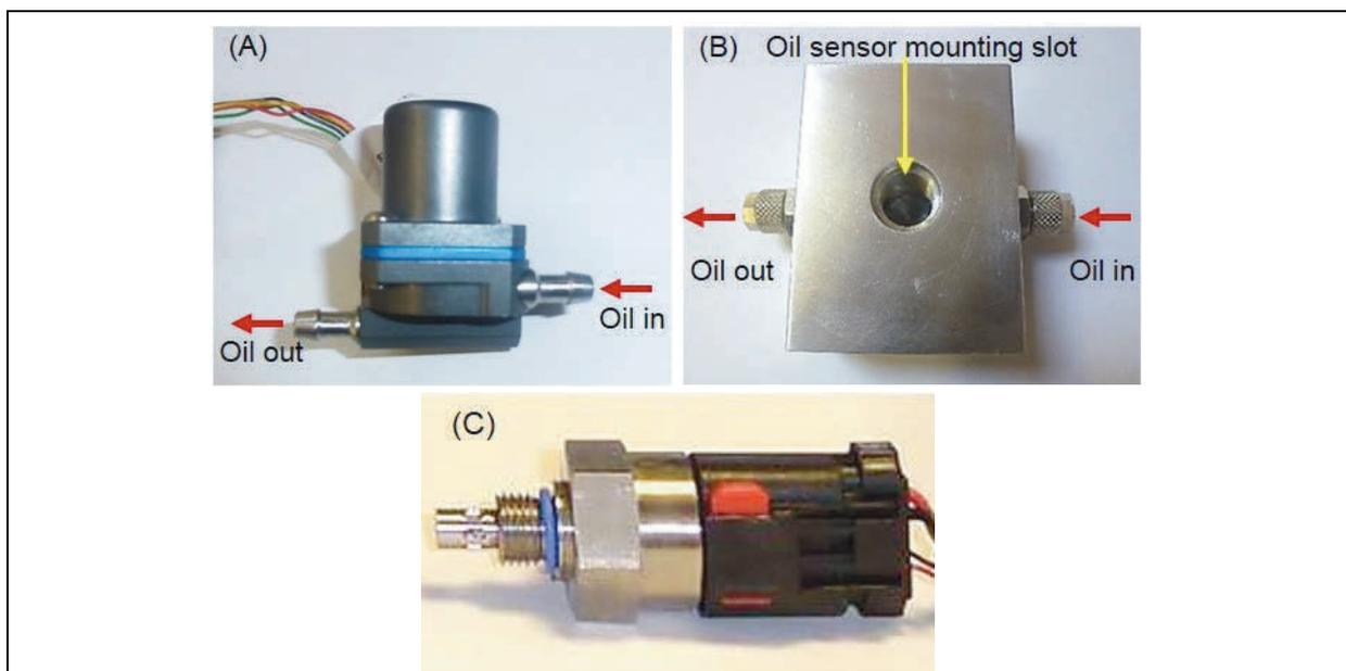
Figure 2: Equipment used in experimental test set-up as (A) Micro-pump, (B) Oil sensor mount and (C) Tuning fork technology based oil sensor
