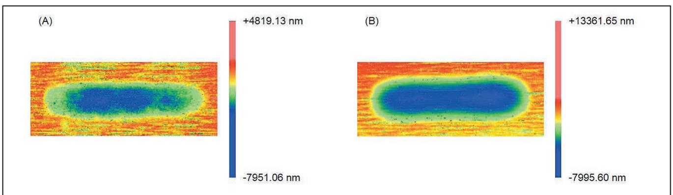
Figure 7: Wear scar on flat plate samples after tribo-testing with (A) oil sample 2 and (B) oil sample 3
