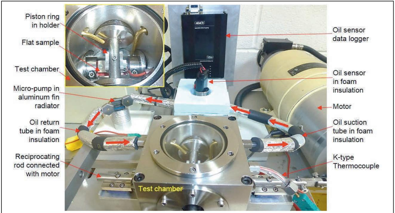
Figure 1: Illustration of experimental test set-up showing oil sensor connected with tribometer
