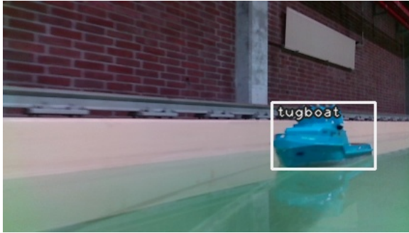
Figure 3: Example Obstacle Detection Output - The resultant bounds and classification of the detected obstacle are annotated on the input image.
