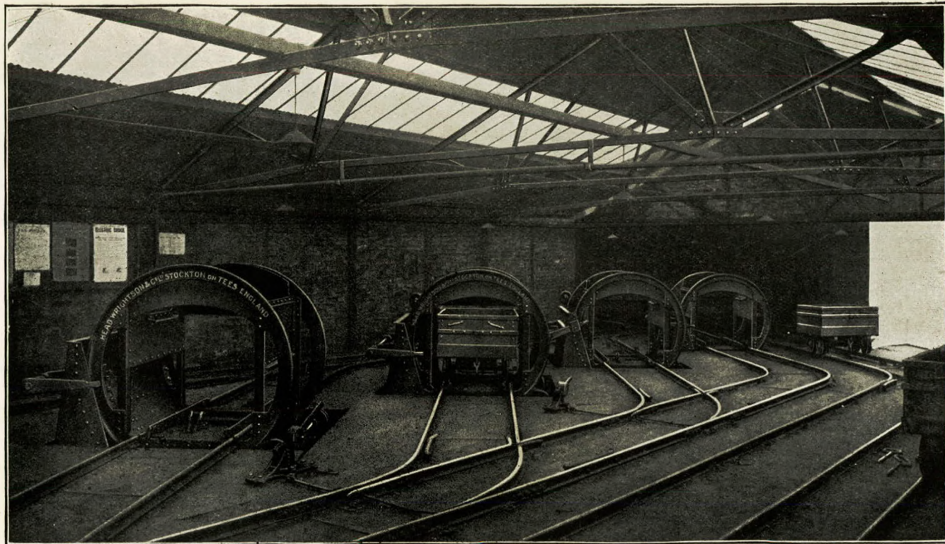
482.—Friction driven tipplers arranged at an angle to their respective screens.
