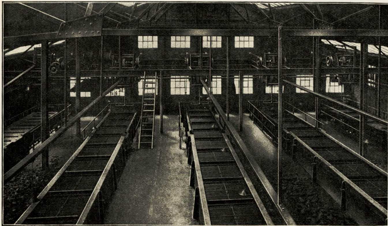
485.—Overhead gears for raising and lowering the deflecting ends of the belts so that coal is lowered to the bottom of the wagon with the minimum of breakage.
