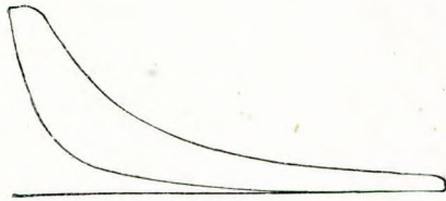
Fig. 64. Diesel Full Load Diagram.
