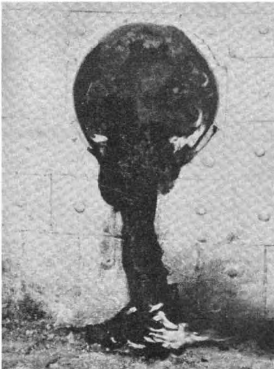
FIG. 2.—(ABOVE) FLAME FROM ADMIRALTY CLOSED FRONT REGISTER AFTER CARBON DEPOSITS HAVE BUILT UP ON THE BRICK TUBE.
