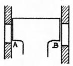
narrower than that at B, the velocity of the steam through A will tend to be higher, thus lowering the pressure locally with the result that there is an unbalanced pressure which forces the valve against one side of its cylinder and friction will prevent it from closing completely.
