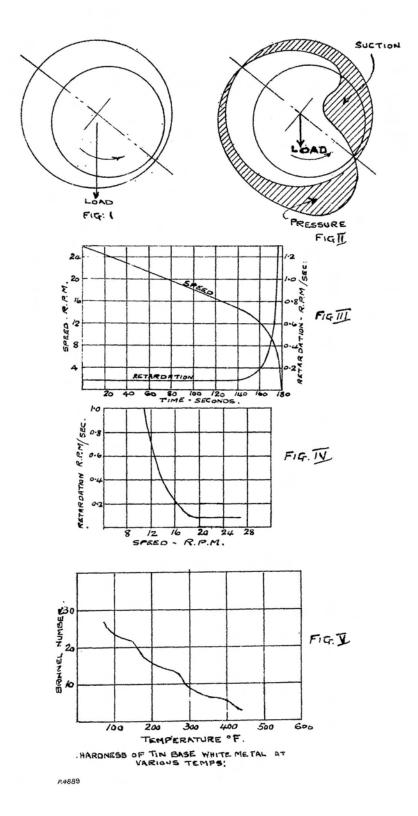
It was formerly common practice to make the bearing length not less than  $1\frac{1}{2}$  to 3 times the diameter, but modern bearings are often not so long as their diameter. Modern practice for turbine bearings, etc., where reversing loads are not imposed, tends to larger clearances, from  $1\frac{1}{2}$  to 3 thousandths of an inch per inch diameter being usual, the larger clearance ratios being used for smaller bearings.
