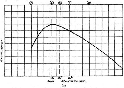
A.F.O. 2080/26 and the accompanying sketch is of interest in connection with the question of air supply. For maximum efficiency of combustion we see that ((x) is the ideal air pressure, and that with either more or less air pressure the efficiency falls off—much more steeply towards "A" due to incomplete combustion than towards "B" (too much air pressure).
