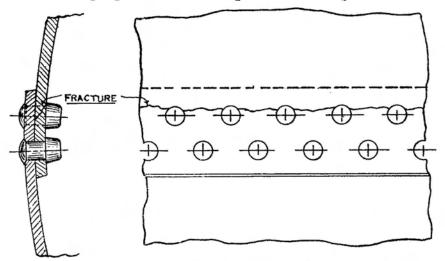
longitudinal seams were situated in the steam space and were ell above the normal water-level maintained in the boiler. The two seams of the end strakes of plate were on one side of the drum and the centre strake seam diametrically opposite.
