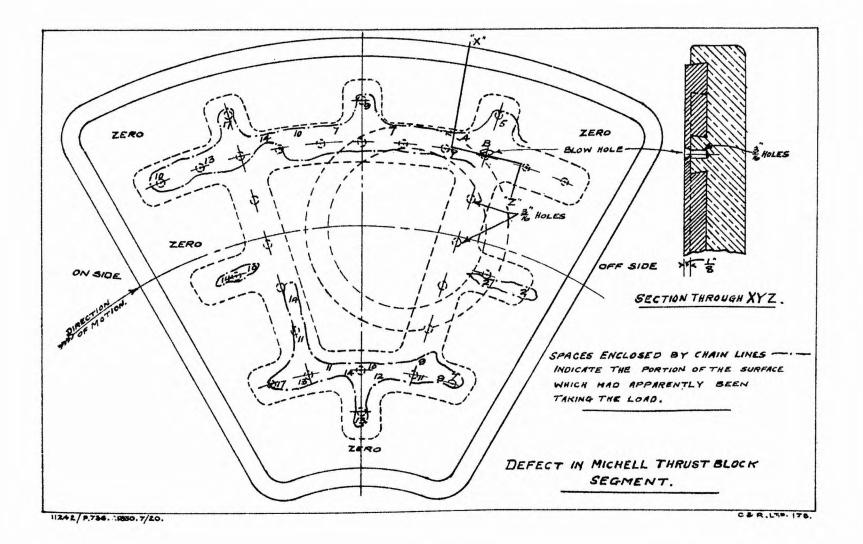
In the execution of her duty, the vessel took another in tow, and the defects became evident when a speed of revolution of 250 per minute had been attained. The evidence showed that the ship's staff had not appreciated that under these towing conditions the full designed pressures on the engine bearings were being realised and possibly somewhat exceeded. No steps had been taken to increase to an adequate extent the oil supply or to apply any cooling water, with the result stated.
