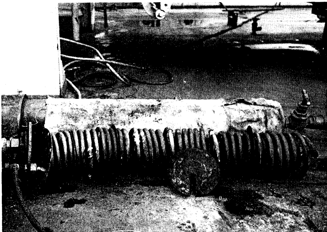
THE HEATING COILS AS ORIGINALLY FITTED
