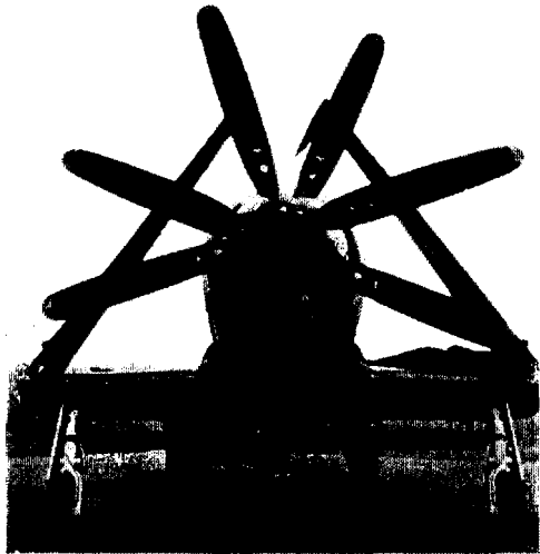
WYVERN PROPELLER IN FINE PITCH SHOWING LARGE BLADE FRONTAL AREA
