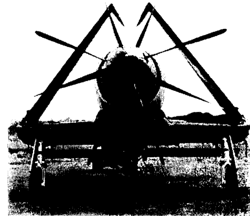
WYVERN PROPELLER "FEATHERED" SHOWING REDUCED FRONTAL AREA AND CONSEQUENT DRAG REDUCTION
