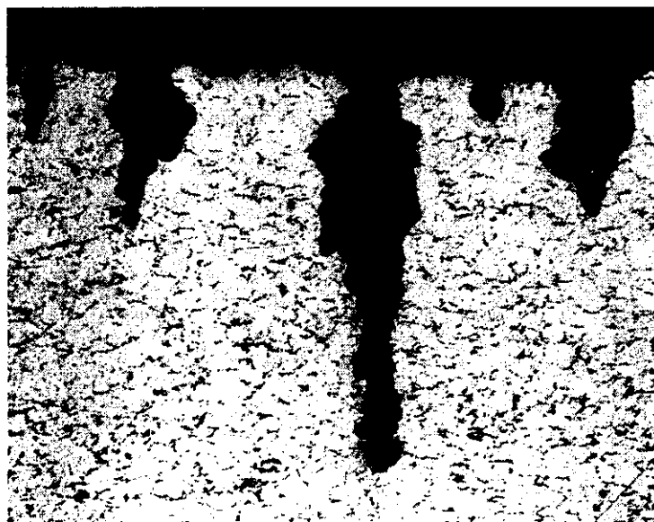
FIG. 22—TYPICAL CRACK IN A28 SHOWING OXIDE ON SIDES AND ABSENCE OF SHARPNESS NOTED IN FIG. 18. THE SPHEROIDIZED MICROSTRUCTURE MAY BE NOTED
