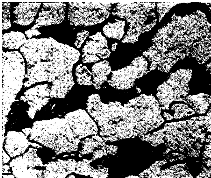
FIG. 3—PHOTOMICROGRAPH OF NORMAL STRUCTURE OF TUBES NOS. 6 AND 7. THIS IS A MIXTURE OF PEARLITE AND FERRITE—USUAL FOR AN APPROXIMATELY 0.25 PER CENT CARBON STEEL (400 ×)
