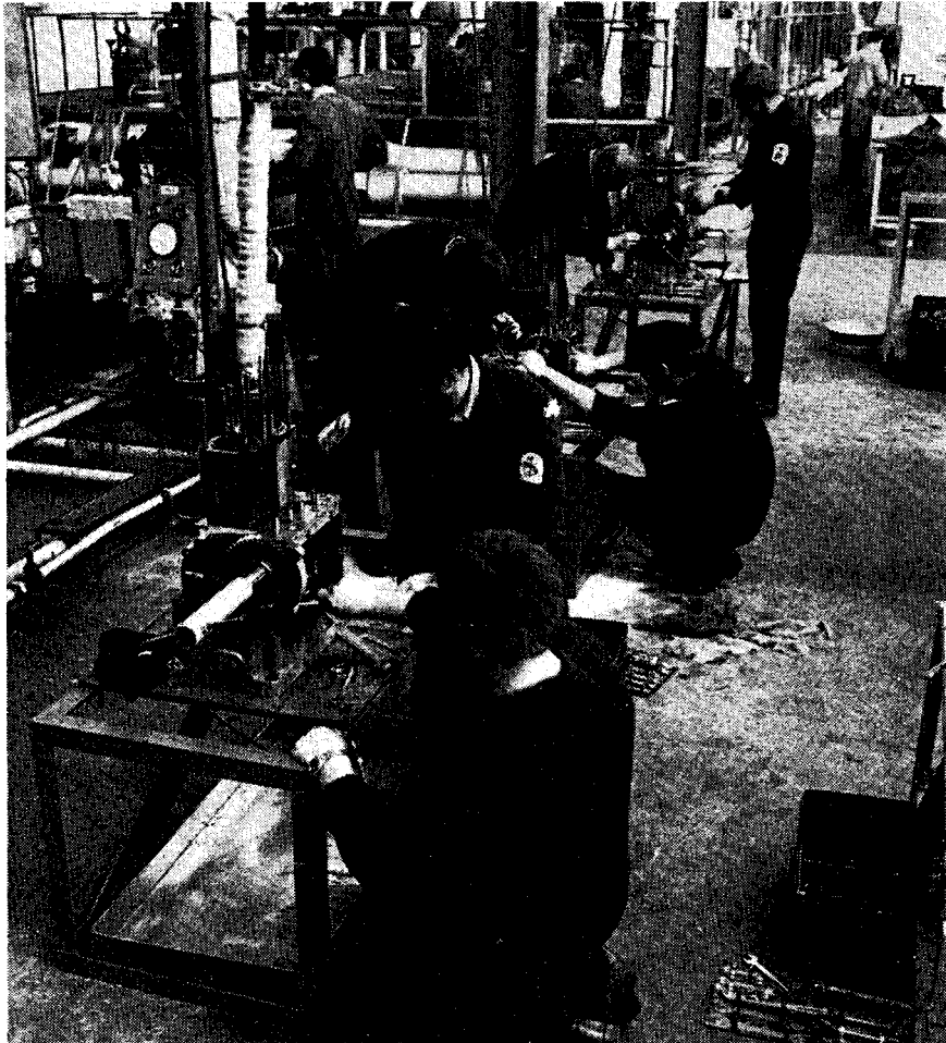
FIG. 4—LMEMs AND POMEMs ENGAGED ON PRACTICAL OVERHAUL OF LISTER SR2 MOTOR-BOAT ENGINE DURING THE SBD COURSE
