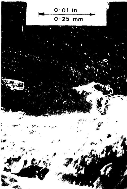
FIG. 4—CRACKING, SPALLING, AND PITTING ON SURFACE OF DRIVEN FLANK OF TOOTH
