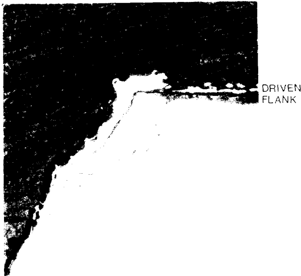
FIG. 5—SECTION OF TOOTH SHOWING CRACKING BETWEEN DRIVEN FLANK AND FRACTURE FACE
