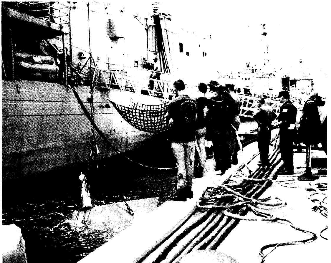
FIG. 6—RED TEAM SUPERVISE THE REMOVAL OF USS 'DOYLE'S' PORT FIN STABILIZER
