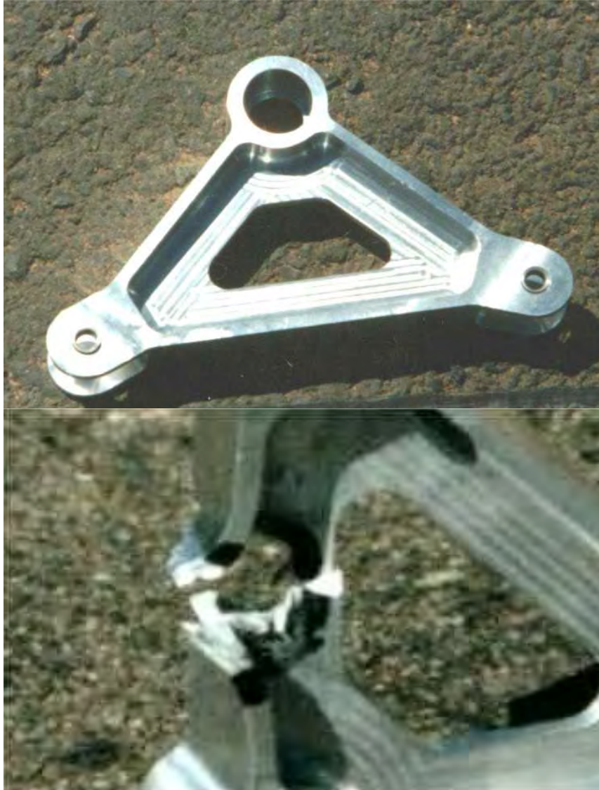
FIG.8 – DAMAGE-TOLERANT FLYING CONTROL LEVER (BELL-CRANK) WITH REDUNDANT LOAD-PATH, BEFORE AND AFTER DAMAGE FROM 12.7 MM AP BULLET (source: author)
