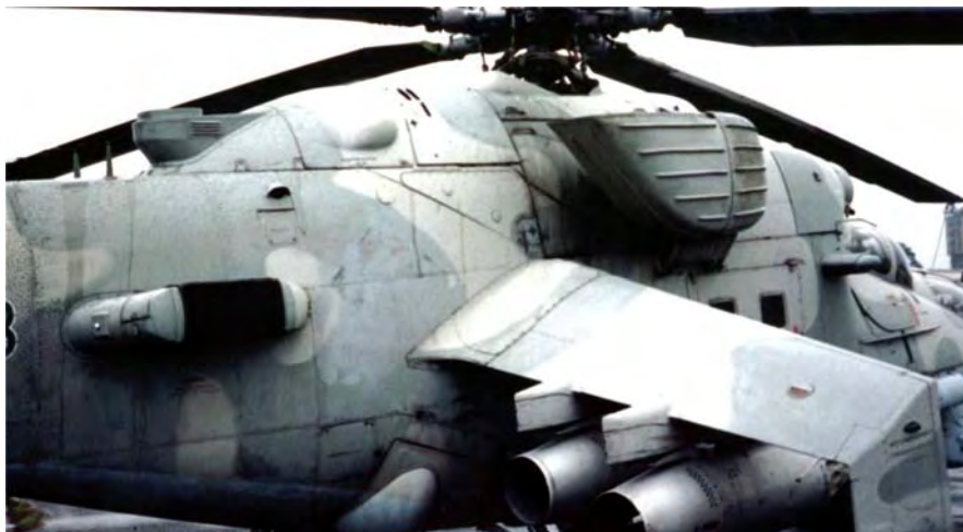
FIG.3 – MIL.24 HIND, ILLUSTRATING THE MEASURES TAKEN TO REDUCE SUSCEPTIBILITY TO IR GUIDED MISSILES. NOTE THE IR JAMMER IS NOT FITTED BUT THE MOUNTING PLATFORM FOR IT IS CLEARLY VISIBLE. (source: author)
