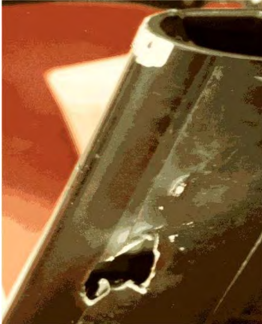
FIG.10 – DAMAGED MAIN ROTOR BLADE (SOURCE: AUTHOR)
