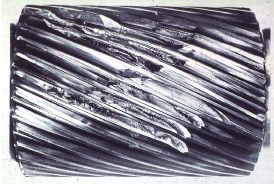
FIG.3 – SSN PRIMARY PINION FAILURE
