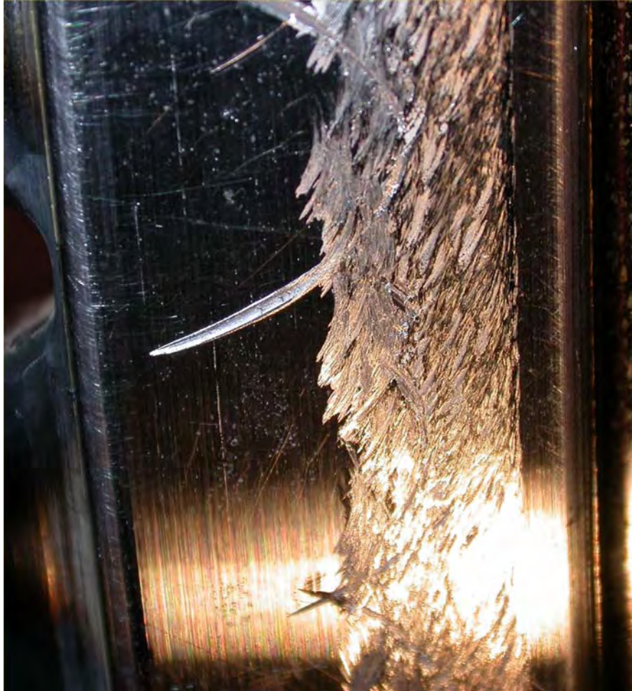
FIG.8 – HMS LANCASTER THRUST CONE DAMAGE
