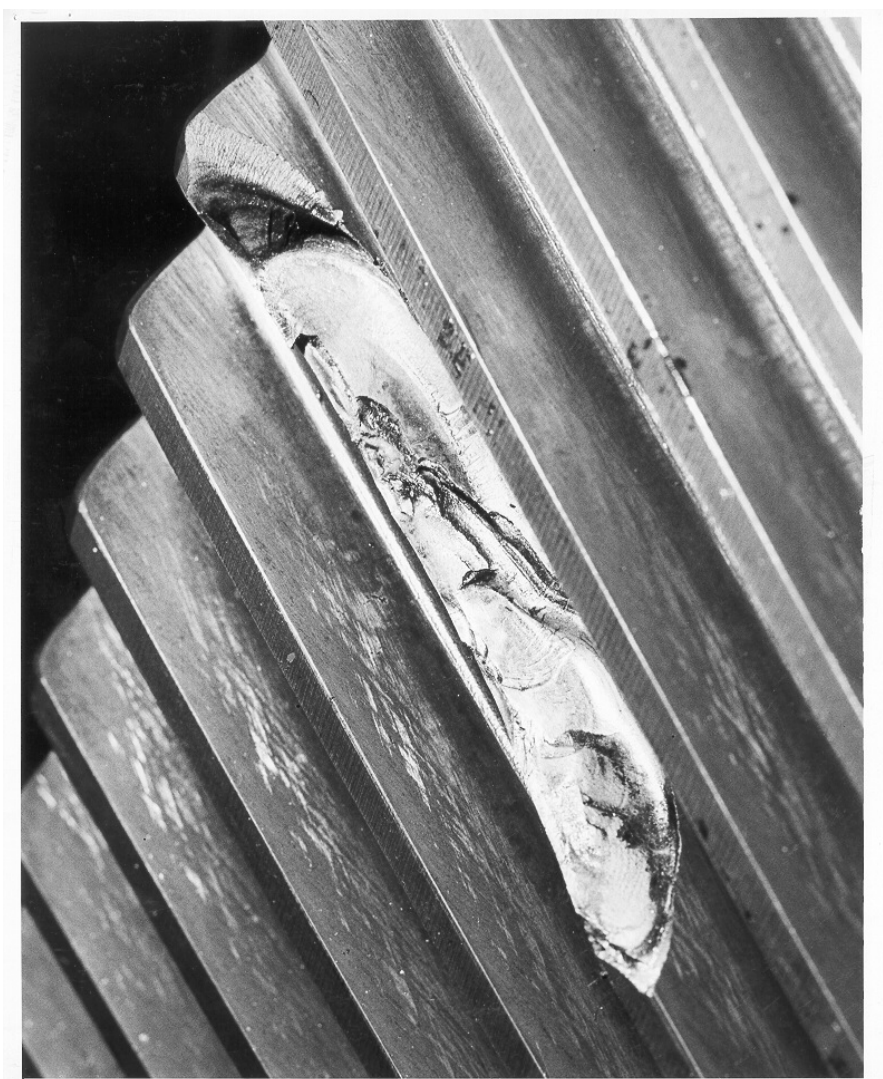
FIG.2 – CVS BROKEN PRIMARY WHEEL TOOTH
