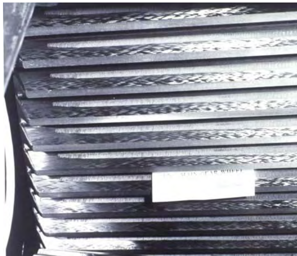
FIG.4 – HMS VANGUARD SECONDARY GEAR SCUFFING
