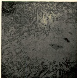
Slide No. 15. Mild Steel Thrust Shaft at fracture. 58 diameters. \text{NH}_4\text{NO}_3 .
