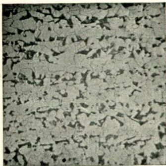
Slide No. 1. Mild Steel. 58 diameters. \text{HNO}_3 .
