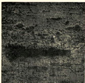
Slide No. 2. Wrought Iron Stay. 53 diameters. \text{HNO}_3 .
