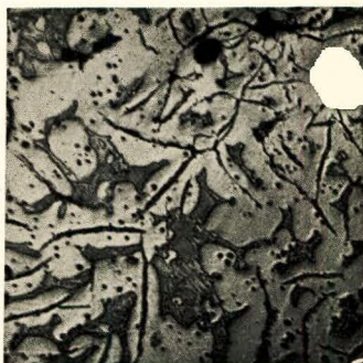
Slide No. 27. Phosphoretic Cast Iron. 75 diameters. Heat tinted.
