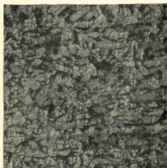
Slide No. 10. Mild Steel Boiler Plate, normal. 53 diameters. \text{NH}_4\text{NO}_3 .
