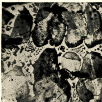
Slide No. 28. Phosphoretic Cast Iron. 236 diameters. \text{HNO}_3 .
