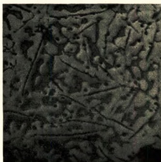
Slide No. 1b. Cleveland Pig-iron. 58 diameters. Heat tinted.
