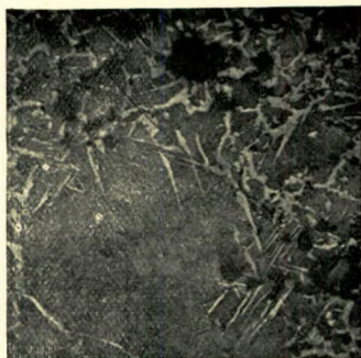
Slide No. 21. Metal found inside a forging. 24 diameters. \text{NH}_4\text{NO}_3 .
