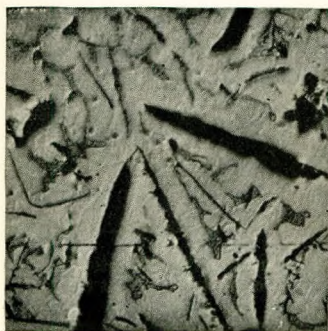
Slide No. 31. Carron Pig-iron. 53 diameters. Heat tinted.
