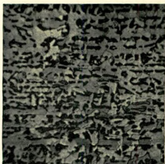
Slide No. 9. Mild Steel Boiler Plate, near centre. 58 diameters. \text{HNO}_3 .
