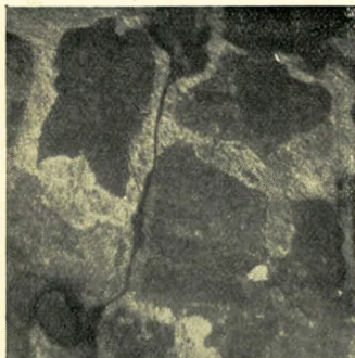
Slide No. 22. Metal found inside a forging. 236 diameters. \text{NH}_4\text{NO}_3 .
