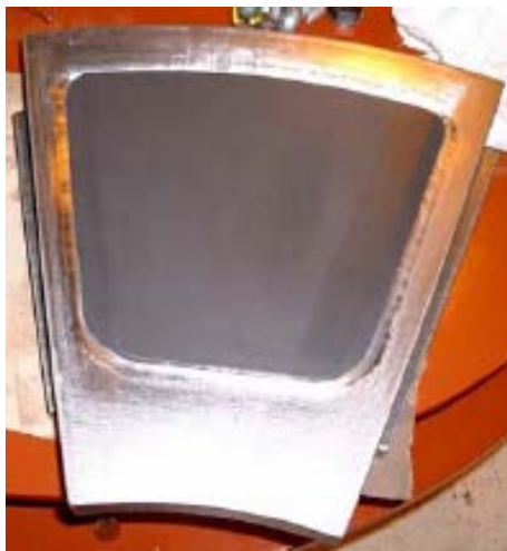
FIG.3 - PTFE THRUST PAD USED IN RIG [1]
