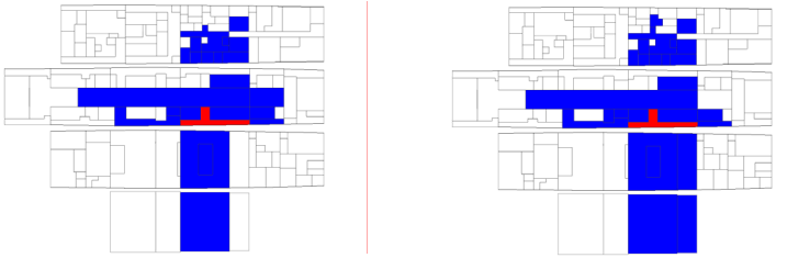
FIG.16 - COMPARISON OF ACTUAL (LEFT) AND SURVIVE PREDICTION OF BLAST SPREAD ON EX-HMS DEVONSHIRE
