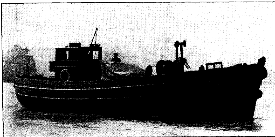
FIG. 3.—45 FT. M.F.V. WITH CHRYSLER ROYAL PETROL OR ATLANTIC 6 B.E. DIESEL ENGINES 60 H.P. SINGLE SCREW. 14 TONS CARGO OR 100 PASSENGERS.
