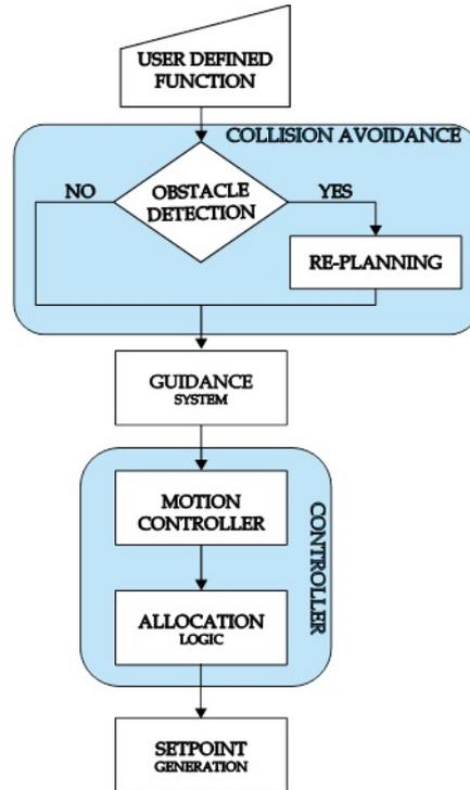
Figure 15: Control structure of the UNIGE's autonomous vessel.
