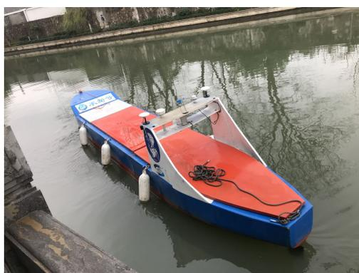
Figure 20: A 7m KVLCC2 model ship.
