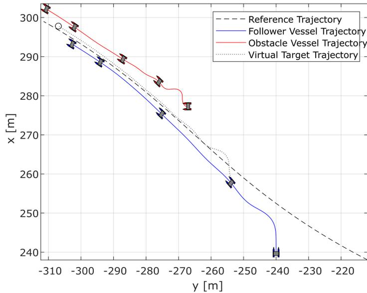
Figure 10: Trajectory of the follower and obstacle vessel following a virtual target
