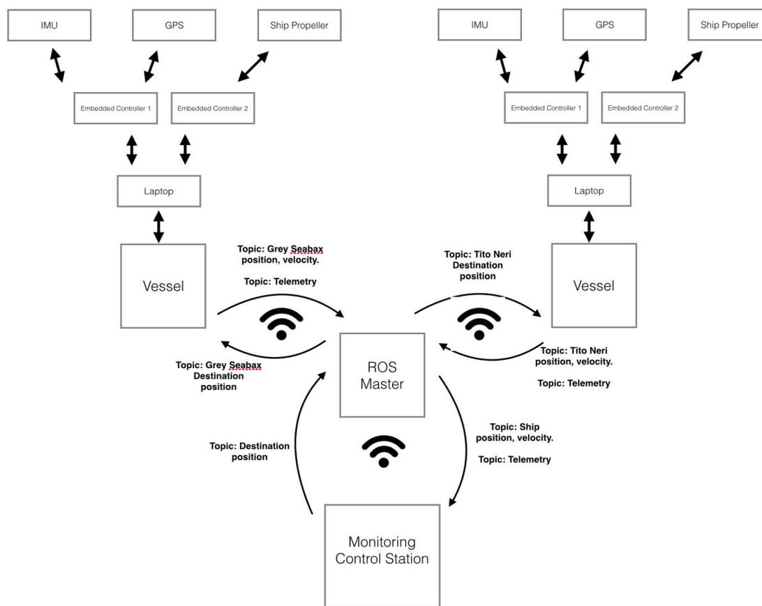
Figure 25: Conceptual block diagram of the control structure.
