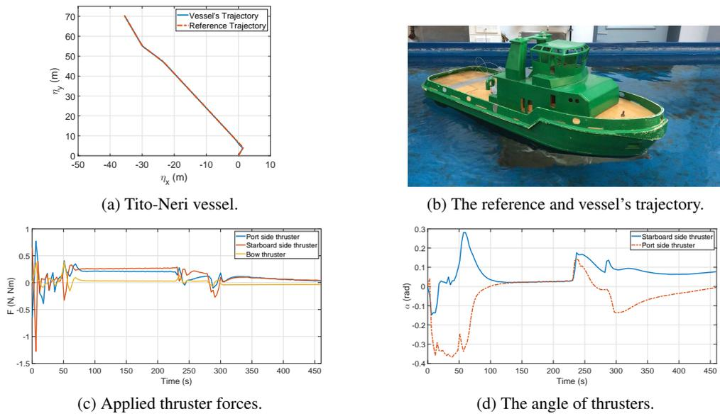
Figure 21: Model predictive trajectory tracking performance of Tito-Neri.
