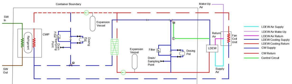
Figure 7 – Schematic Representation of a Containerised Modular LDEW Cooling System
