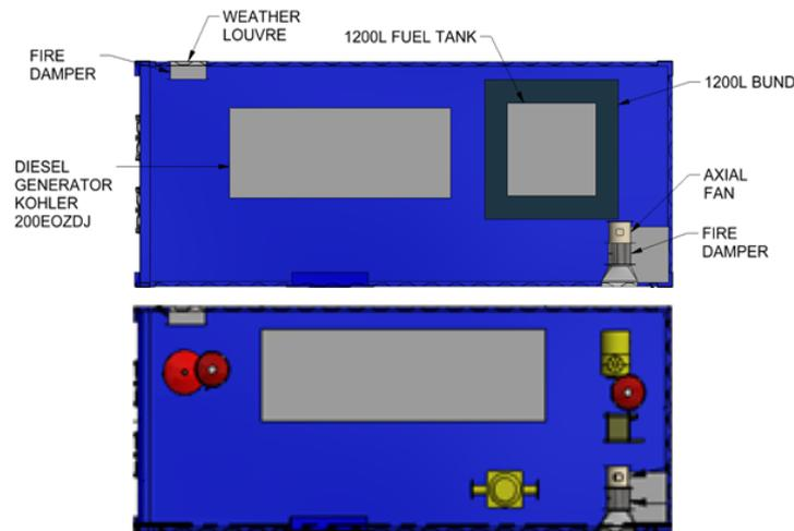
Figure 10 – Plan View of 2 x 20ft. ISO Containers Incorporating Power Generation and Chilled Water Plant
