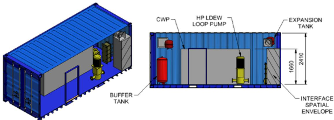
Figure 9 – 20ft. ISO LDEW Cooling Container Incorporating Chilled-Water Plant
