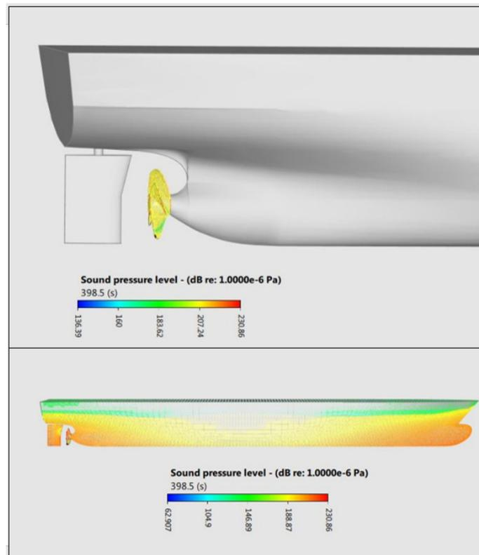
Figure 6(a)Top: Hydrodynamic pressure computed from CFD mapped on propeller; Figure 6(b) Bottom: Hydrodynamic pressure computed from CFD mapped on hull, propeller and rudder surface
