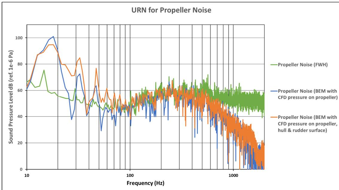
Figure 8 URN from propeller as a noise source for various numerical models
