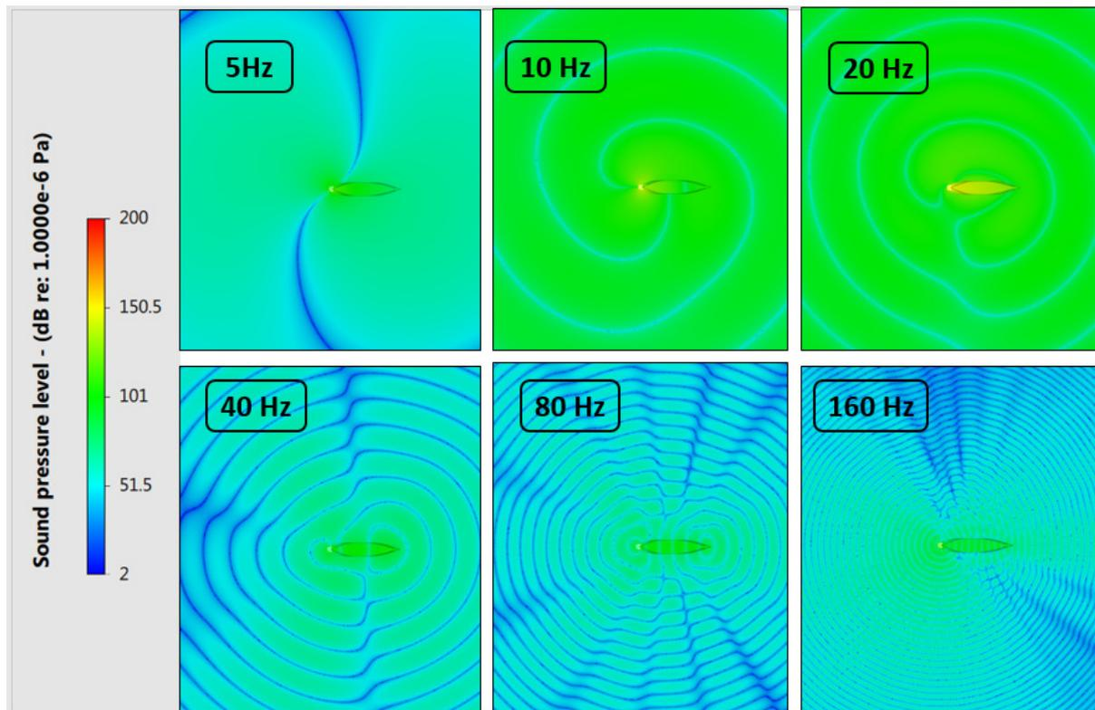
Figure 7. Sound propagation pattern at various frequencies using BEM for propeller noise including scattering effect
