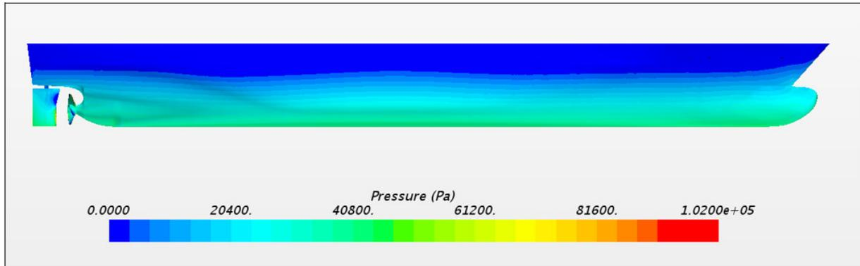
Figure 5: CFD Computed Pressure Field on the hull, propeller and rudder at an instance
