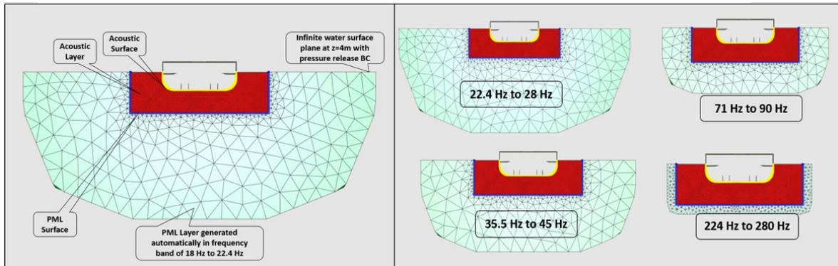
Figure 2(a) Left: PML model for Main Engine Room; Figure 2(b) Right: Adaptive PML generated for various frequency bands
