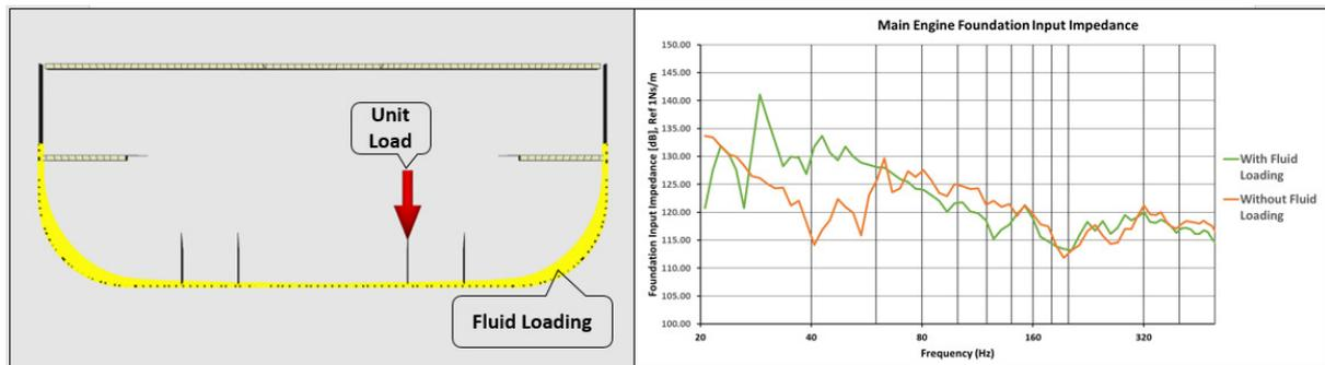
Figure 4(a) Left: ME room section; Figure 4(b) Right: ME foundation input impedance
