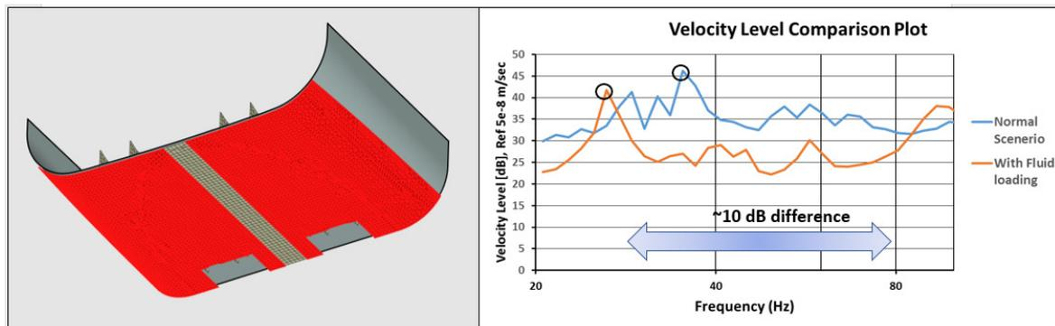
Figure 3(a) Left: Section of ME room for which Velocity levels recorded; Figure 3(b) Right: Velocity Level Comparison Plot (Blue arrow shows range of frequencies for which approximately 10dB difference in the velocity levels is observed)
