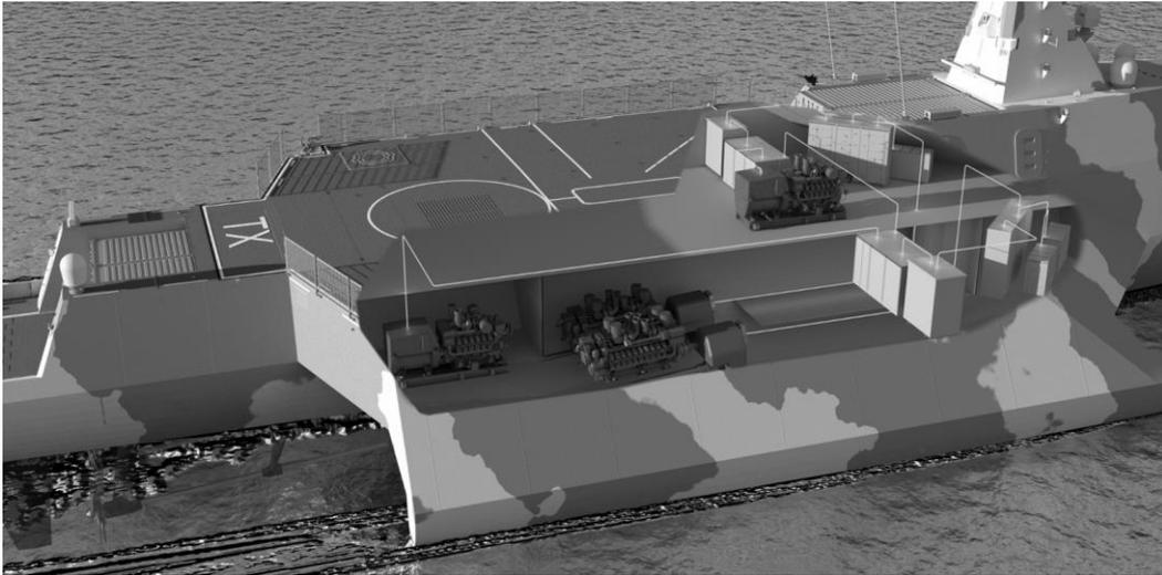
Figure 5 - Illustration of the CODLAD propulsion system within the Tx hull-form
