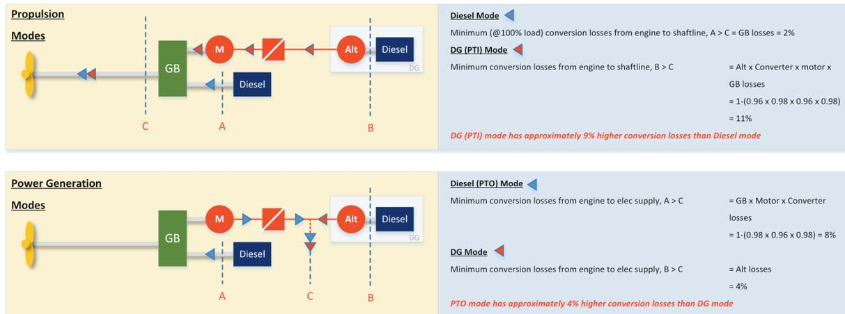
Figure 8- Hybrid Propulsion Modes- Power Conversion Loss Considerations
