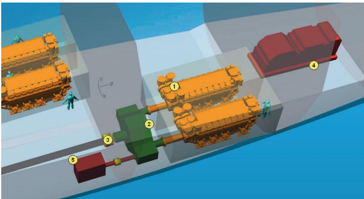
Figure 6- Hybrid VLF Stbd Propulsion Train and Fwd DG
