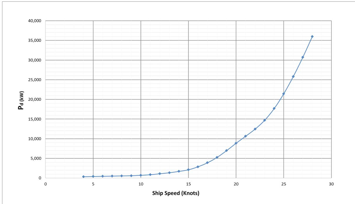
Figure 3: VLF Assumed Power-Speed Curve
