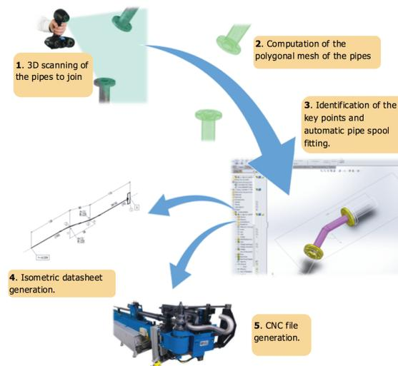
Figure 3. Schematic representation of the five steps involved in the spool fitting tool.
