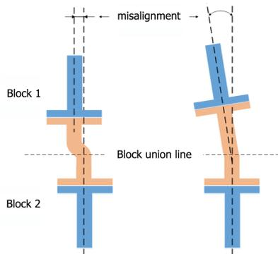
Figure 1. Examples of misalignments: a misalignment due to a non-concentricity of the axes of the pipes to be joined (left pipe), and a misalignment with an angular deviation (right pipe).
