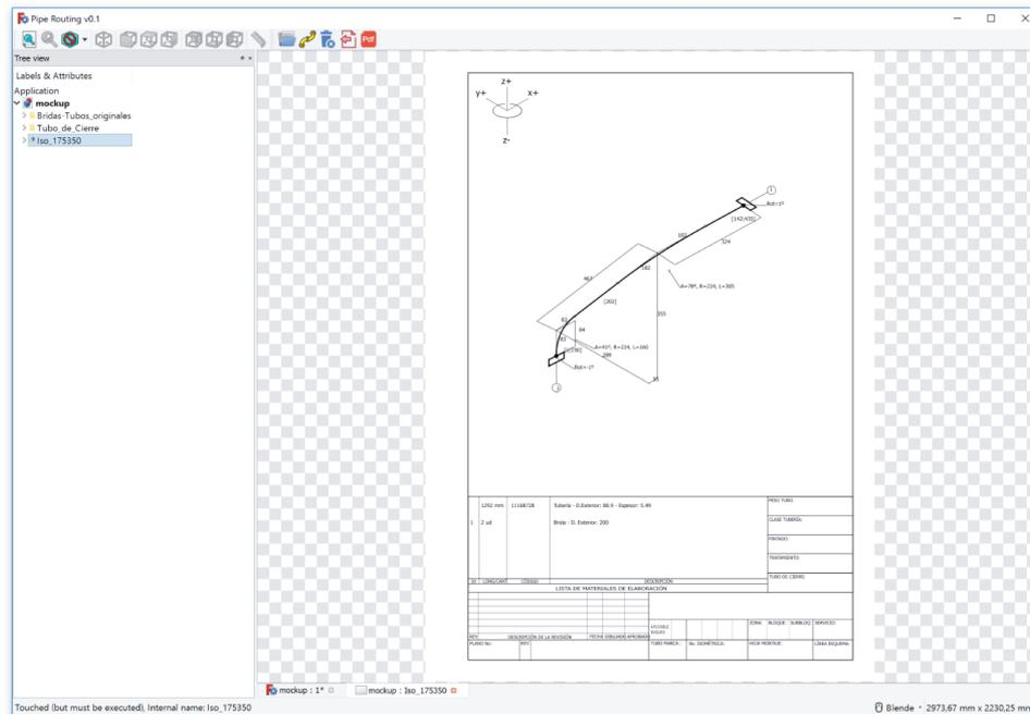
Figure 8. Example of isometric view generated by the software tool.
