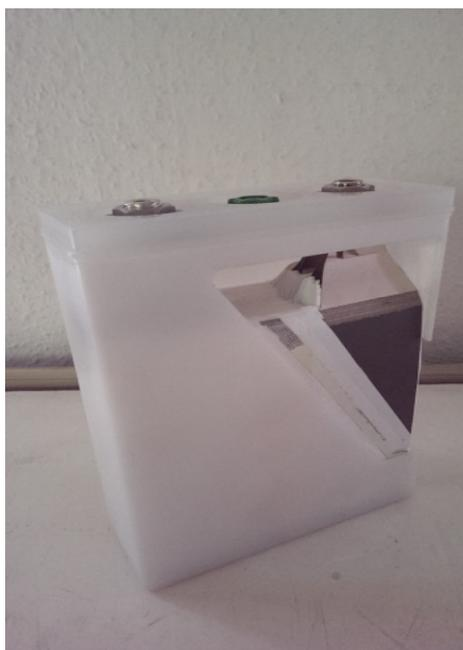
Figure 4. Cut-away view of NiZn cell
