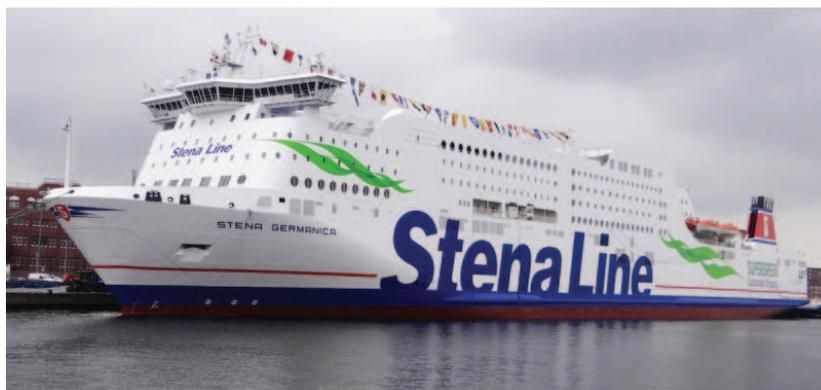
Figure 4: Ro-pax ferry Stena Germanica has been converted to methanol, from (Andersson and Salazar, 2015).
