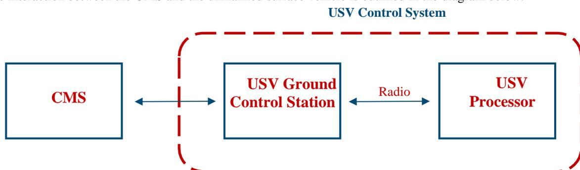
This architecture allows the CMS to send commands to the unmanned surface vehicle’s ground control station which then converts the message to a format readable by the unmanned surface vehicle processor.
