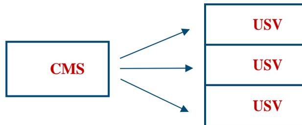
The above scenario would work well when the off-board systems are within good communications range of the mothership. Once out of communication range, the behaviour of the USV will be dependent on the autonomous control software. An example behaviour could be that the USV returns to the last known location where it was receiving communications, known as the Last Response Engine.
