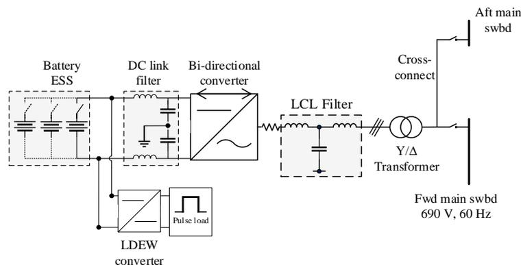
Figure 2: ESS and LDEW integration schematic for half ship set
