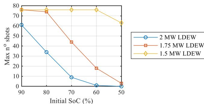
Figure 11: LDEW performance envelope with varying battery SoC
