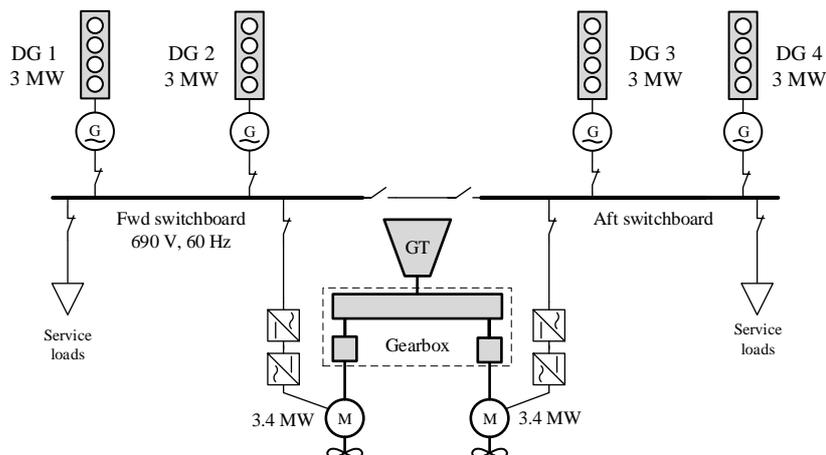
Figure 1: Reference system architecture for case study
