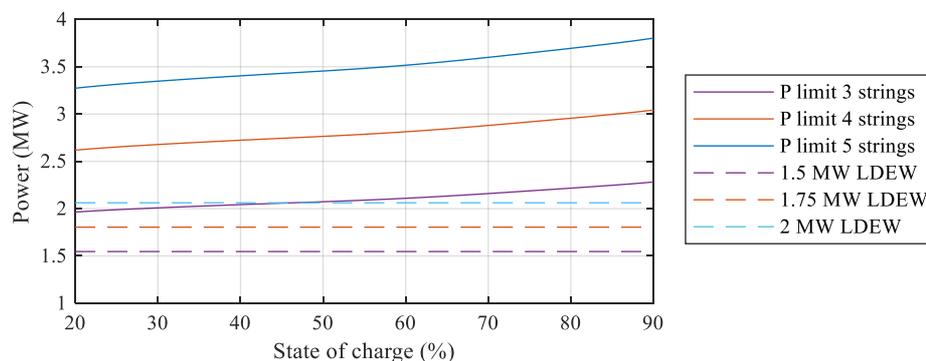
Figure 4: ESS string power limits and LDEW loads of interest- remove LDEW signs
