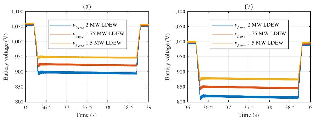
Figure 10: Voltage response to LDEW loading when the simulation commenced at (a) 90% and (b) 70% SoC
