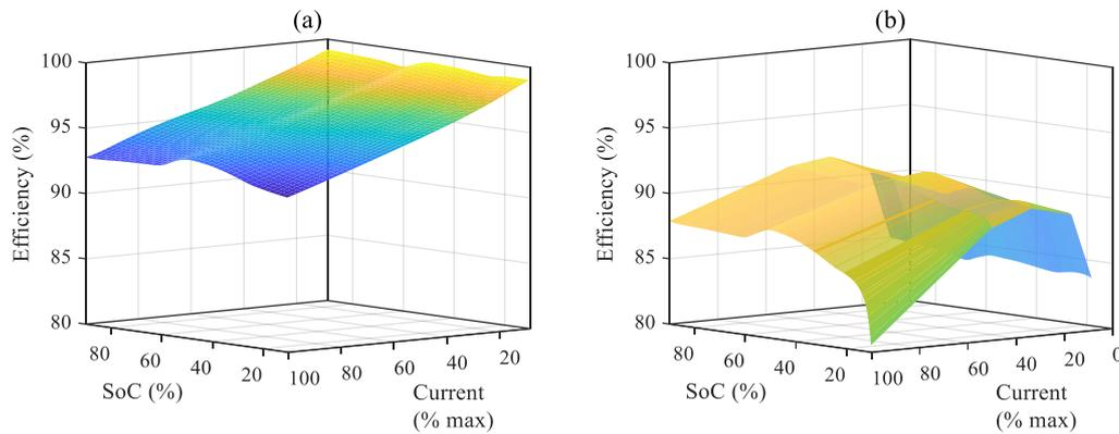
Figure 3: Analytical thermal efficiency map over battery discharge measured at (a) battery terminals i.e. connection to the LDEW converter and (b) connection to the main switchboard
