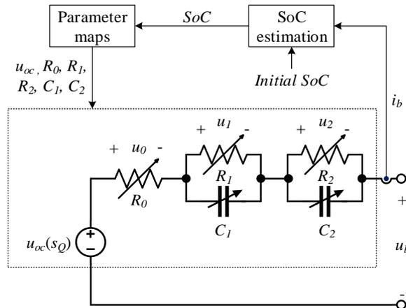
Figure 6: Lithium-ion battery Thévenin equivalent circuit
