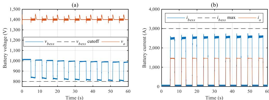
Figure 9: System (a) voltage and (b) current response to 2 MW LDEW load commenced at 70% SoC
