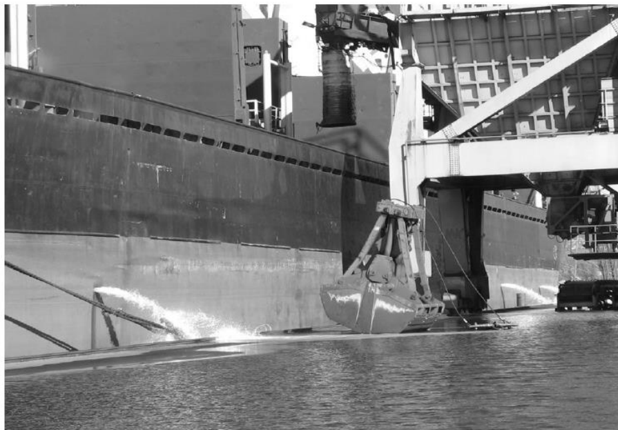
Figure 2. Ballast water discharge above pier level from the upper wing tanks of a bulk carrier. Source: Jure Barovic, with courtesy of the Port of Koper, services for protection of the sea (Consult, 2013)
