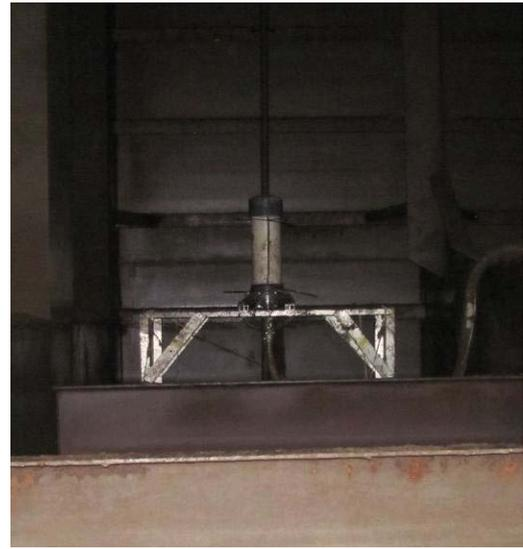
Photo 6 - Point diffuser in tank
