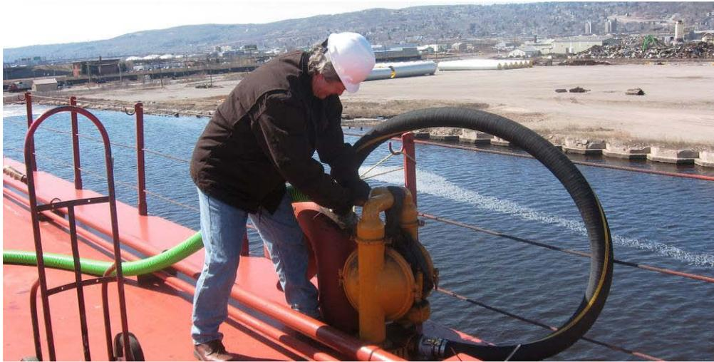
**Photo 20 - Rigging transfer pump and hose on main deck**
