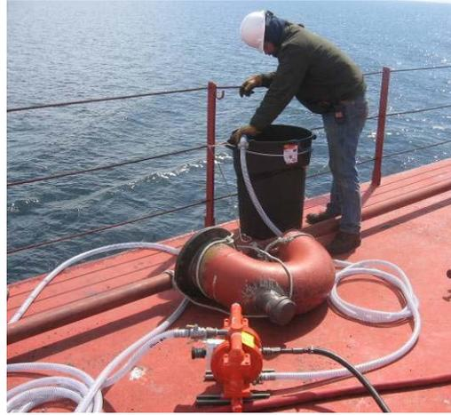
**Photo 10 - Perforated hose setup on deck during dye study**
