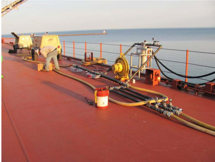
**Photo 18 – Air supply equipment on deck for point diffuser and grid diffuser trials**
