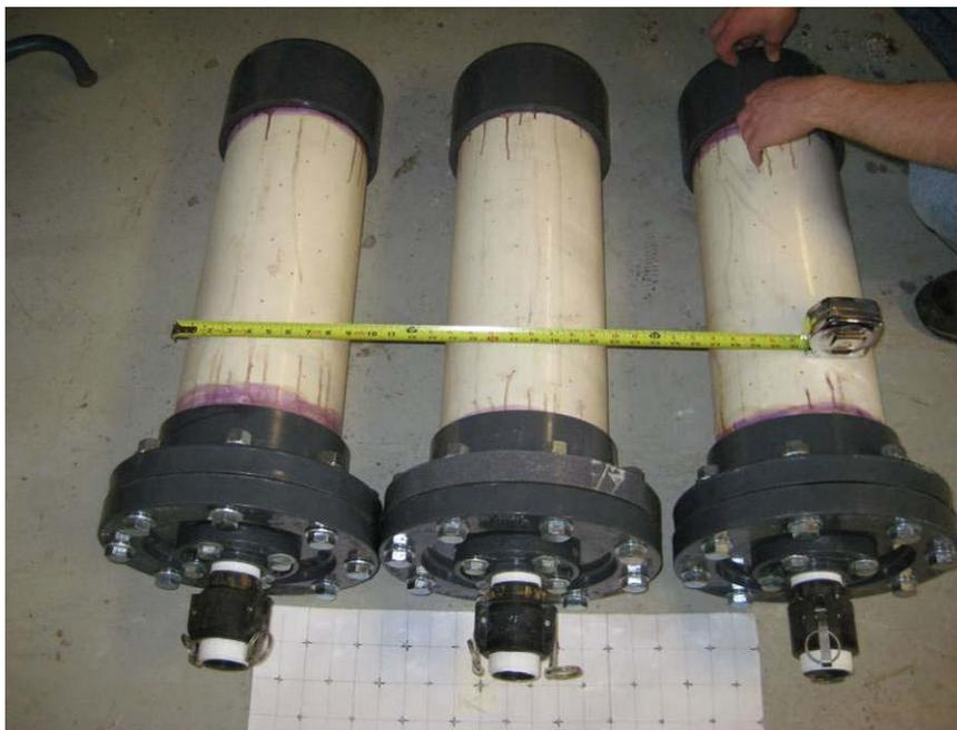
**Photo 16 - Point diffusers, 10" diameter pipes 36" long with ~100 1/8" holes**
