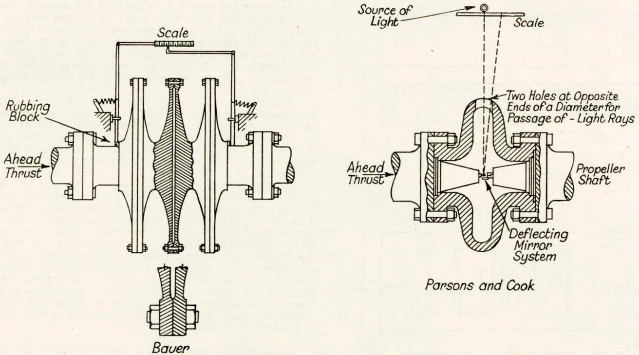
FIG. 14—"Bellows" type thrustmeter
