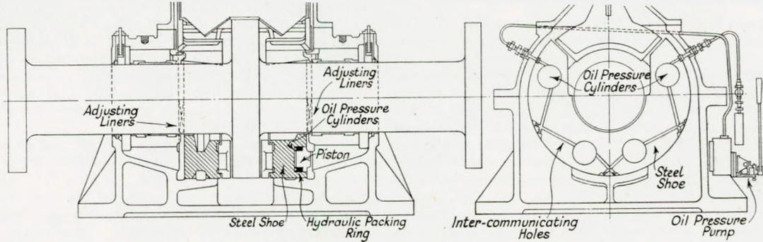
FIG. 11—Michell thrust block with thrust indicator
