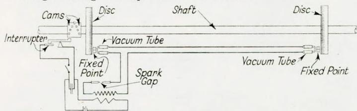
FIG. 2—Stroboscopic torsionmeter
