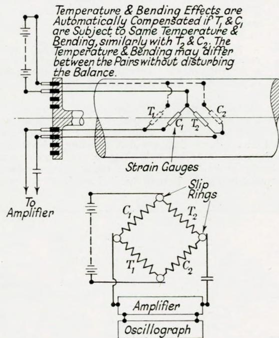
FIG. 10—Wire resistance torsional strain gauge
