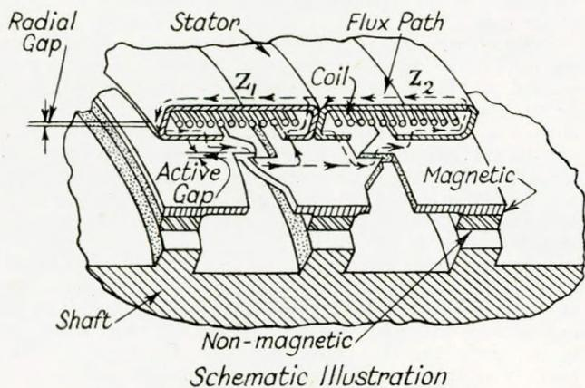
FIG. 7—Magnetic coupled torquemeter
