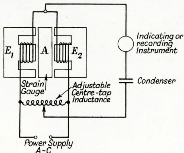
FIG. 16—Westinghouse magnetic strain gauge
