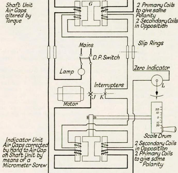
FIG. 5—Schematic arrangement of circuit—Siemens-Ford torsionmeter
