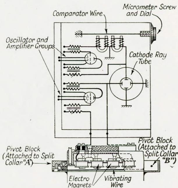
FIG. 3—Maihak torsionmeter. General arrangement and electrical circuit
