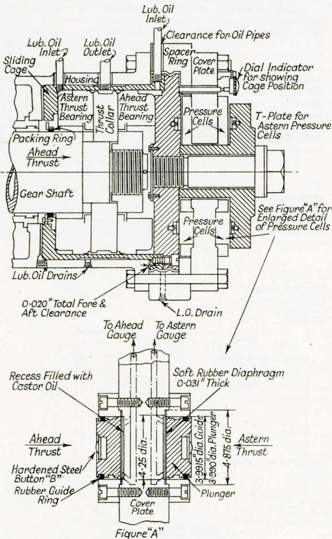
FIG. 13—Kingsbury pressure cell thrustmeter
