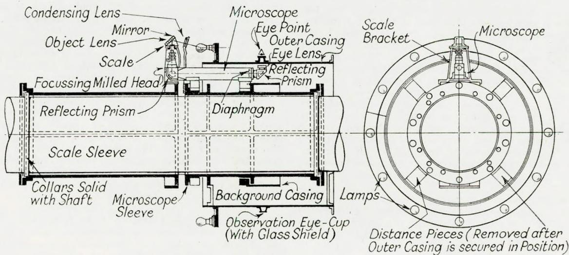
FIG. 1—Denny microptic marine torsionmeter
