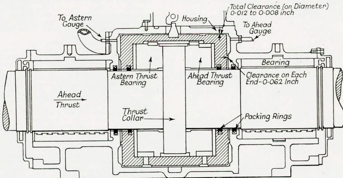
FIG. 12—Westinghouse Electric and Manufacturing Co. thrustmeter
