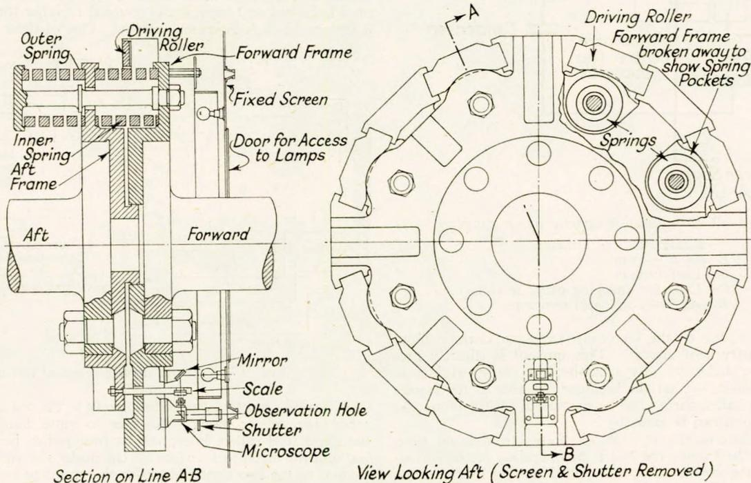
FIG. 15—Denny marine thrustmeter
