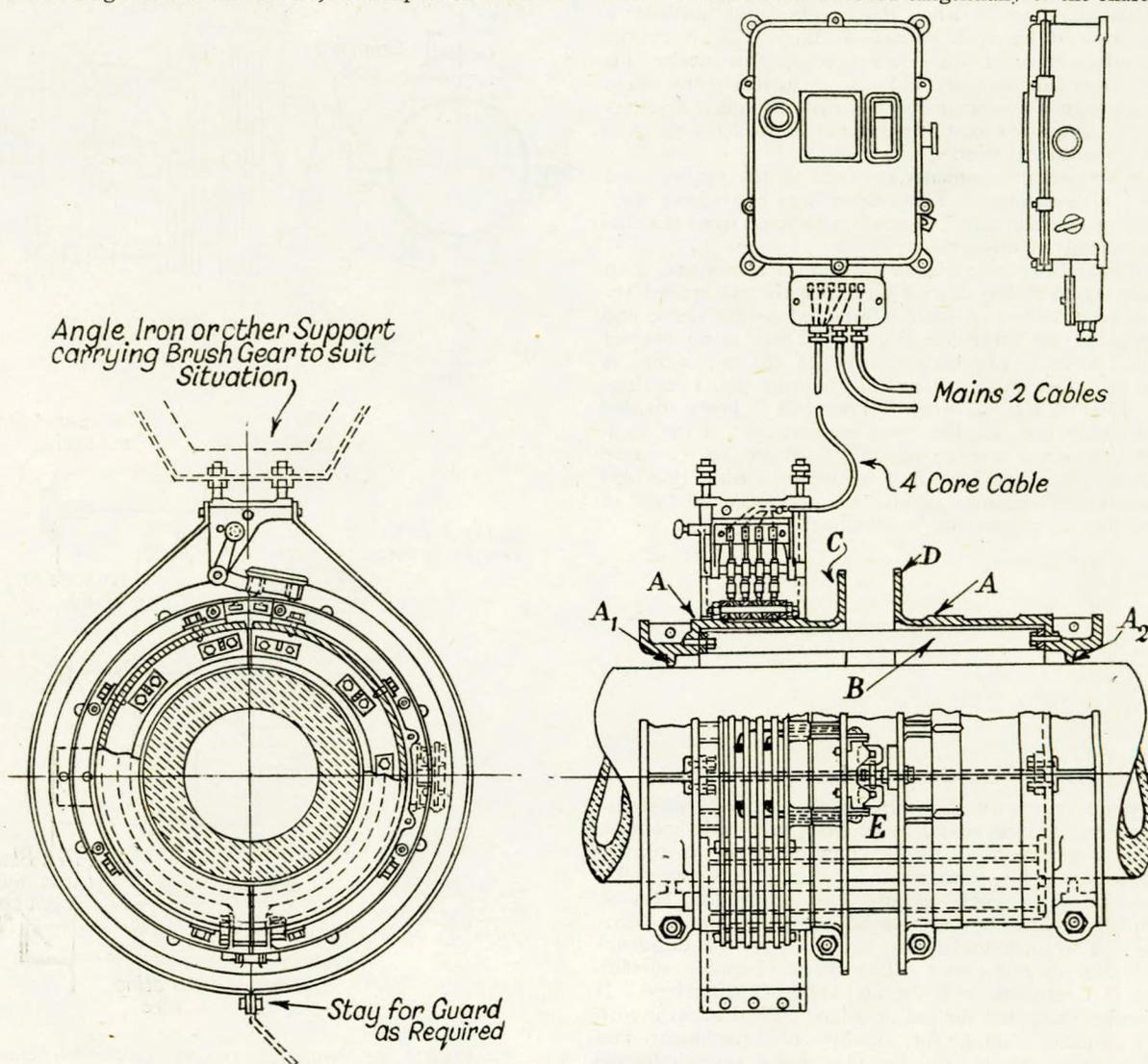
FIG. 4—General arrangement of Siemens-Ford torsionmeter
