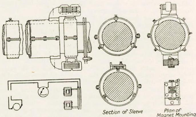
FIG. 6—Moullin torsionmeter
