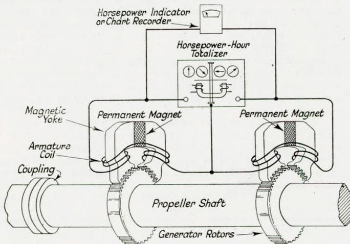
FIG. 9—General Electric of America phase difference generator powermeter
