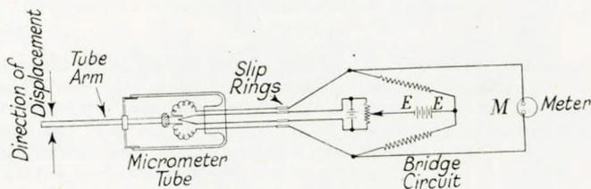
FIG. 8—Micrometer tube (N.R.L.) torsionmeter
