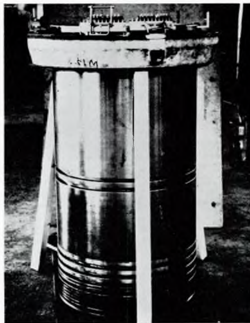
FIG. 32—Exhaust piston with seal ring carrying the contacts
