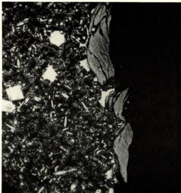
FIG. 21—Micro section through cavitated area, showing iron carbide layers
