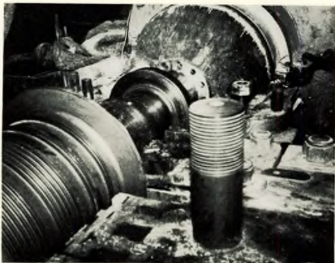
FIG. 14—H.P. thrust collar after first failure
