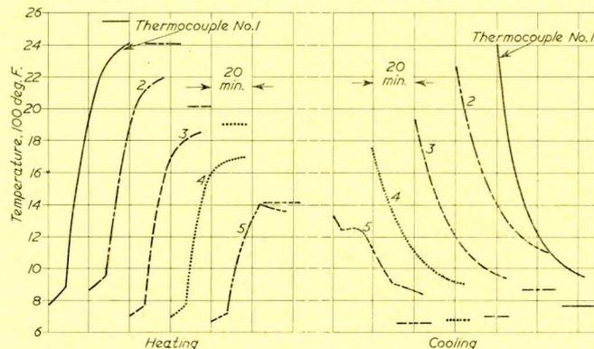
FIG. 14—Heating and cooling curves for points along quarl block, boiler 9
