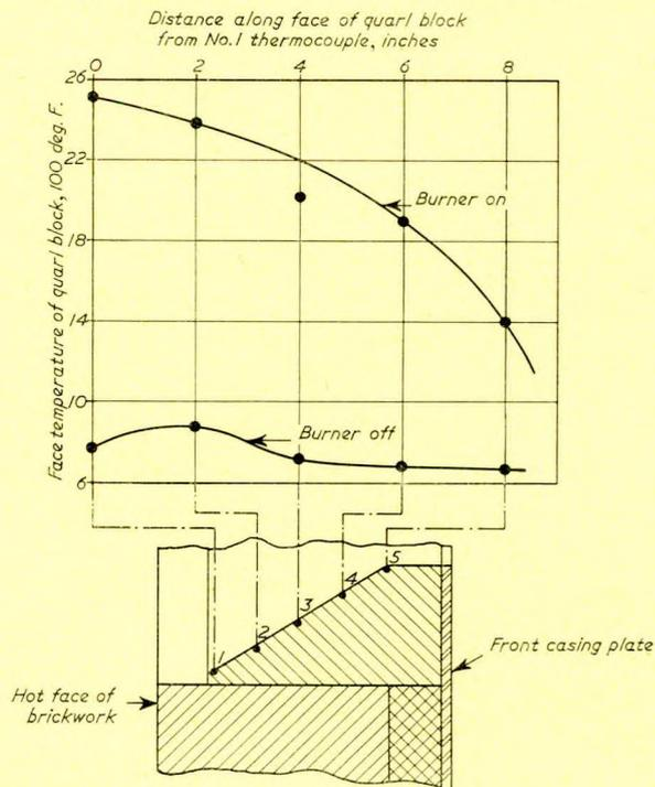
FIG. 15—Steady quarl block face temperatures, boiler 9
