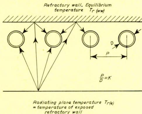
FIG. 6—Diagram illustrating conditions when water wall tubes are fitted
