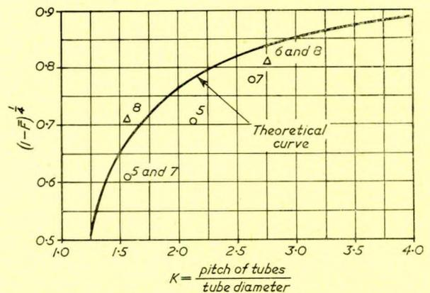
FIG. 7—Effect of tube spacing on reduction in temperature of refractory, compared with exposed wall
