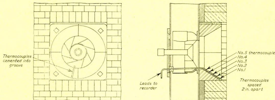
FIG. 12—Arrangement of thermocouples in quarl block, boiler 9
