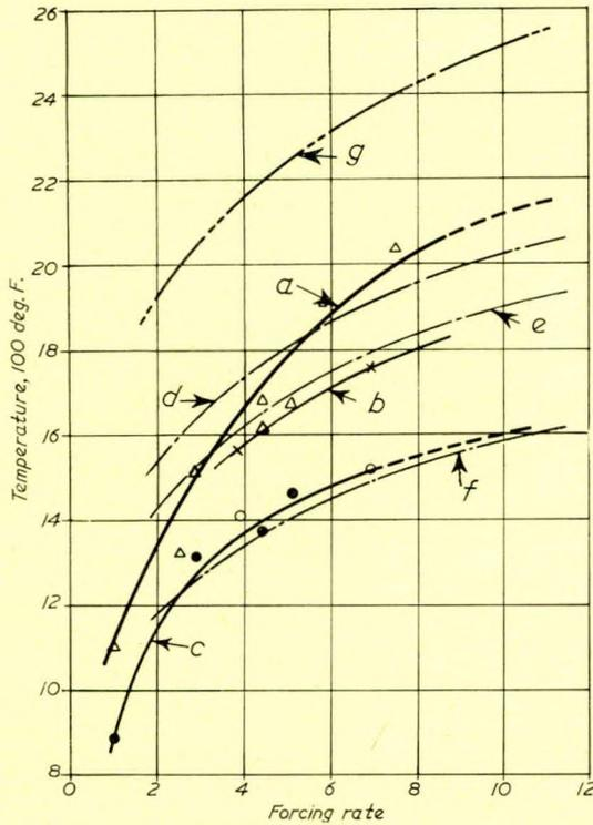
FIG. 9—Effect of water wall tubes on refractory hot face temperature—long flame burners. (Curves drawn for air at 240 deg. F., 2-in. outside diameter tubes)
