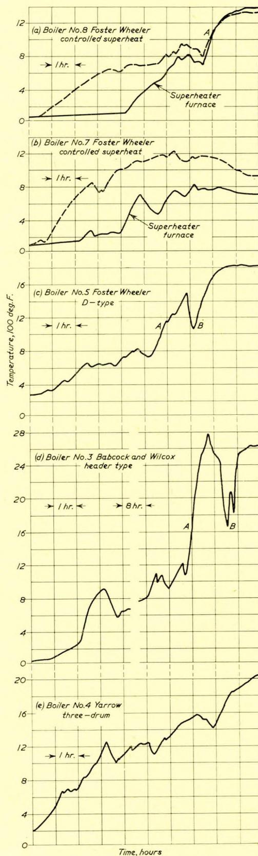
FIG. 11—Typical records of back wall temperatures during steam raising and manœuvring
