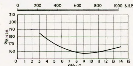
FIG. 1.—Fuel consumption curve for 4-stroke engine with intercooled supercharge
