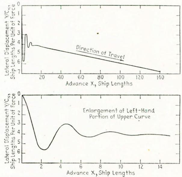
FIG. 29—Course resulting from constant external force and moment—ship "C"
