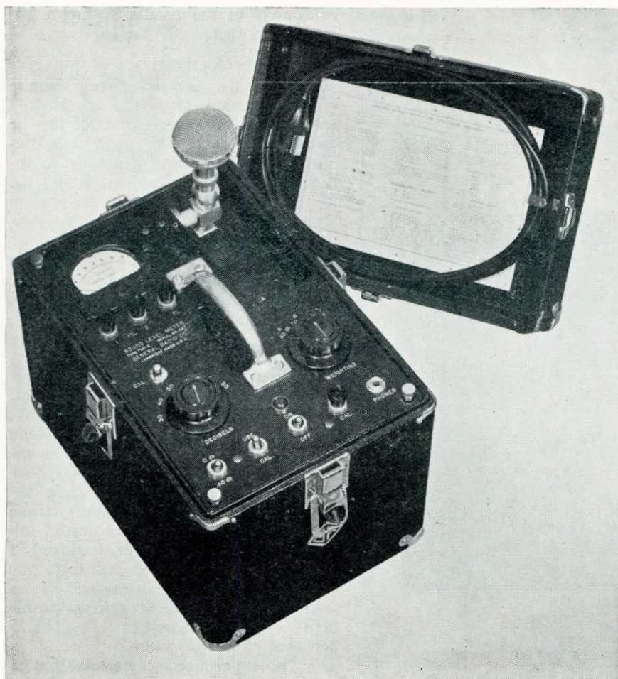
FIG. 3.—Typical sound level meter—objective type.
