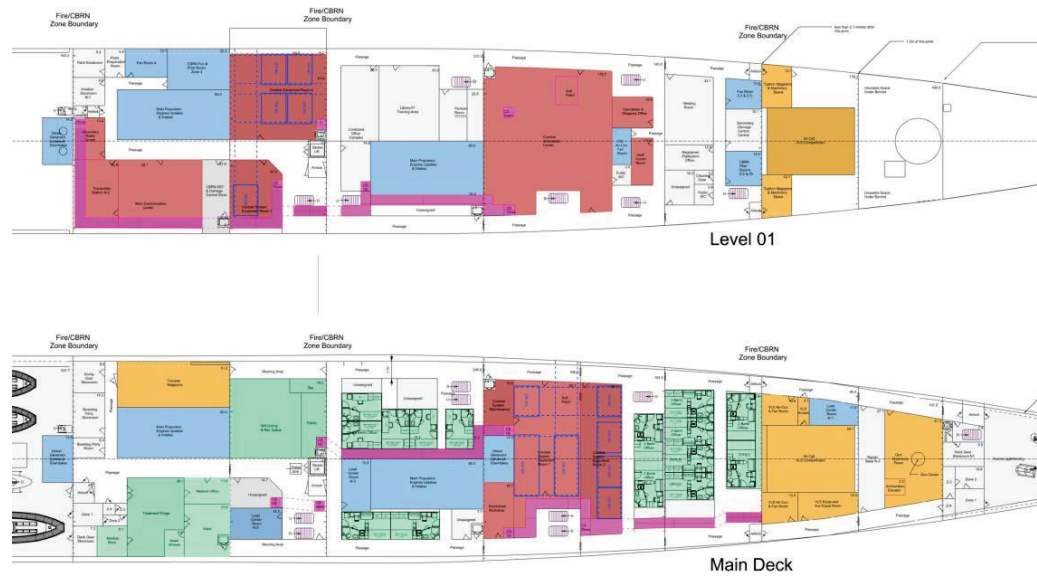
Figure 2: Indicative implementation of combat system enclaves (red) linked by galleries (pink).
