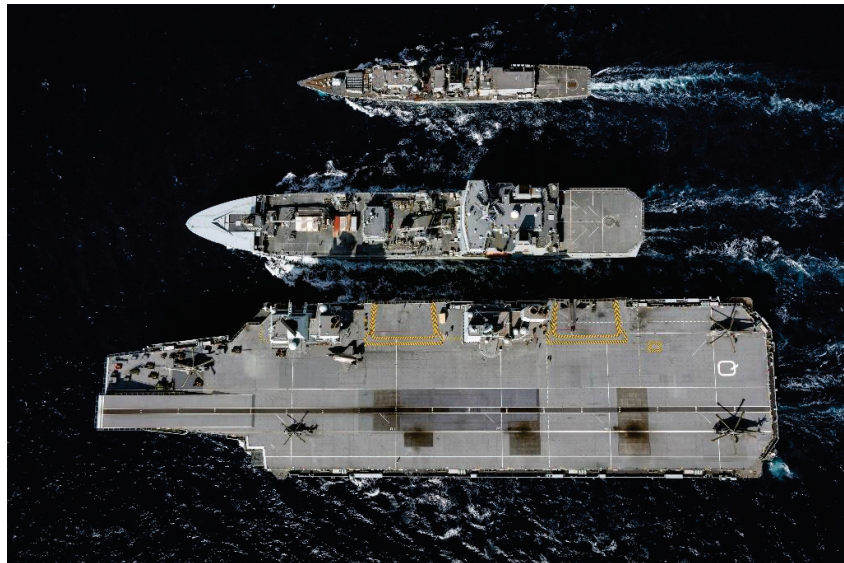
Figure 11 - Cut out the Middle Tanker and Reverse RAS eDiesel from the mother ship to the escorts Credit: © crown copyright 2019
