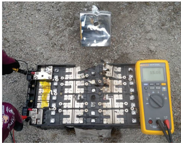
Figure 9 - Overcharge/Overdischarge/Overcurrent/Overvoltage/external short circuit
