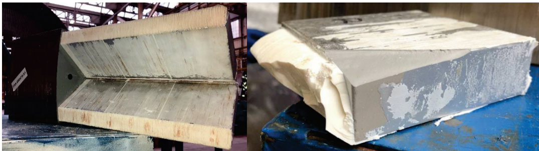
Figure 10: Post test strip-down of test sample: no sign of damage was found on the magnets and rotor components.
