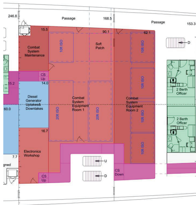
Figure 3: Combat system equipment room modular installation example.
