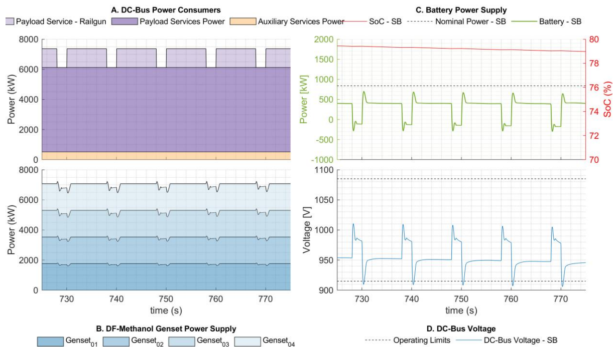
Figure 4-3 PPE performance focussed on railgun recharge operations while sailing in electric mode. Due to limited fast acting sources being available in the electric mode, the designed system is not capable of recharging the railgun for firing at 0.2 Hz. The results for a firing pattern with the railgun firing at 0.1 Hz is simulated.
